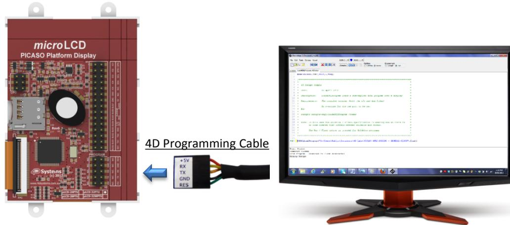
Getting started is as simple as connecting the 4D Programming Cable to the display module, and choosing your product and Development Environment in the 4D Workshop4 IDE.
