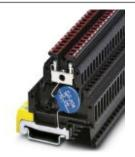
Modular terminal block with varistor as surge voltage protection between clamping connector and DIN rail, separate ground connection, nominal voltage: 12 V AC, mounting on NS 35/7.5, terminal width: 6.2 mm, terminal height: 69 mm
