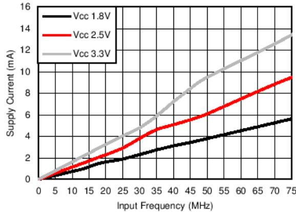
Figure 4. I<sub>CC</sub> vs Frequency
