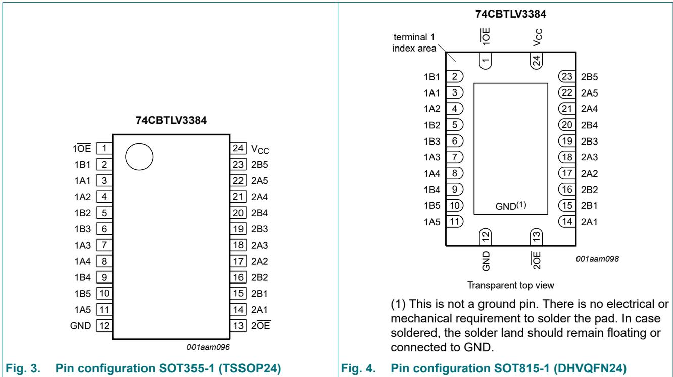
(1) This is not a ground pin. There is no electrical or mechanical requirement to solder the pad. In case soldered, the solder land should remain floating or connected to GND.
