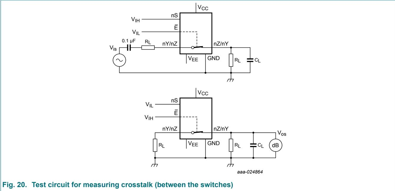
Fig. 20. Test circuit for measuring crosstalk (between the switches)
