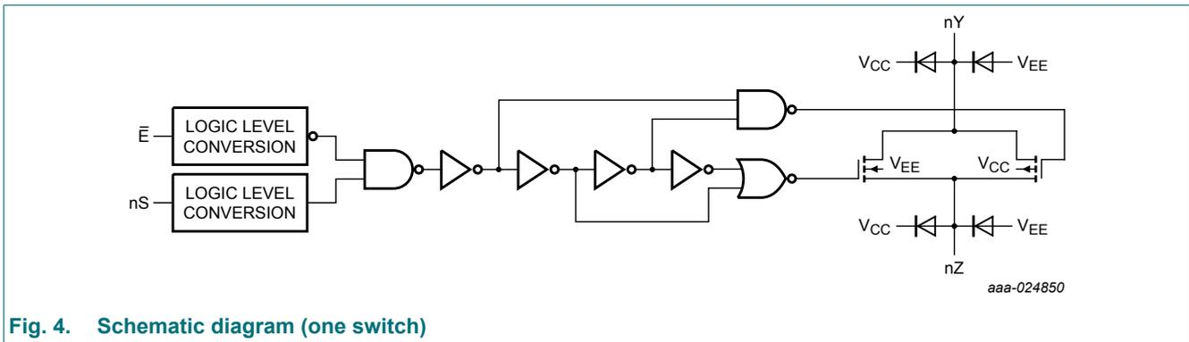
Fig. 4. Schematic diagram (one switch)
