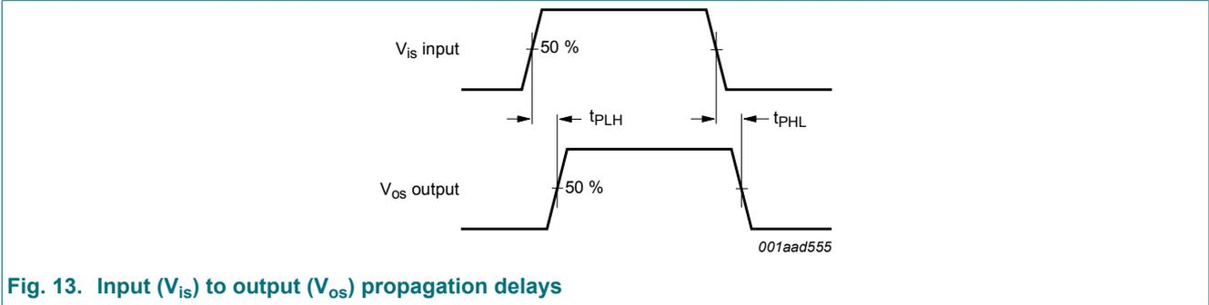
Fig. 13. Input ( $V_{is}$ ) to output ( $V_{os}$ ) propagation delays
