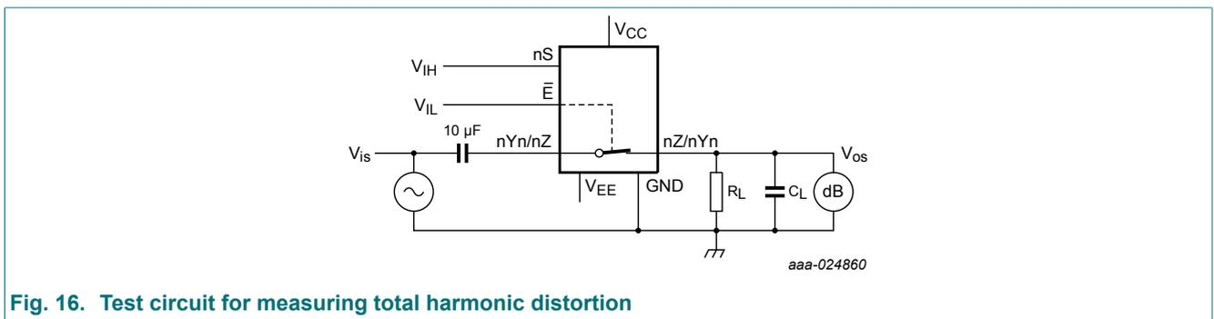
Fig. 16. Test circuit for measuring total harmonic distortion
