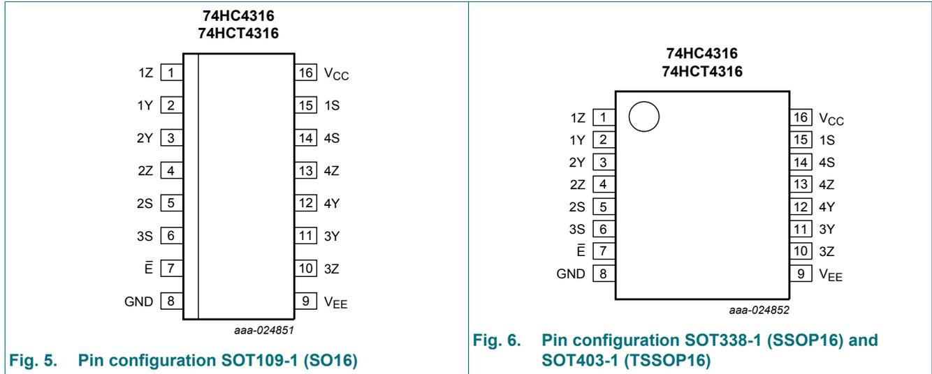
Fig. 5. Pin configuration SOT109-1 (SO16)
