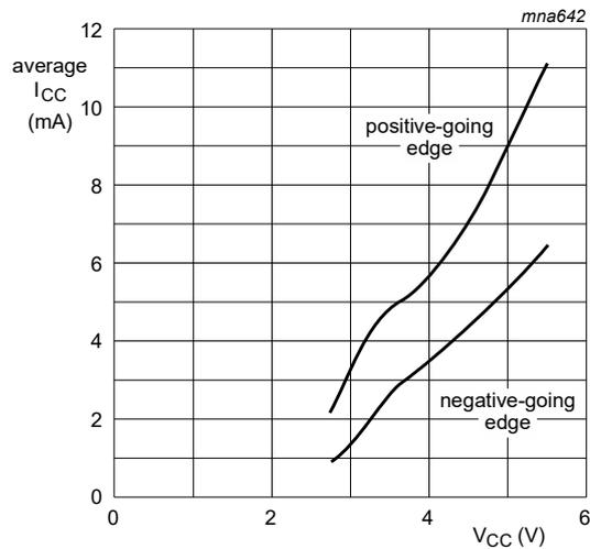
Linear change of  $V_I$  between 0.8 V to 2.0 V.
