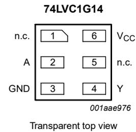
Fig. 5. Pin configuration SOT886, SOT1115 and SOT1202 (XSON6)
