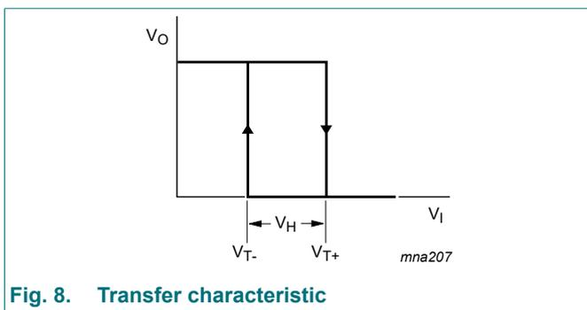
**Fig. 8. Transfer characteristic**
