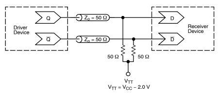
Figure 3. Typical Termination for Output Driver and Device Evaluation (See Application Note <u>AND8020/D</u> – Termination of ECL Logic Devices.)
