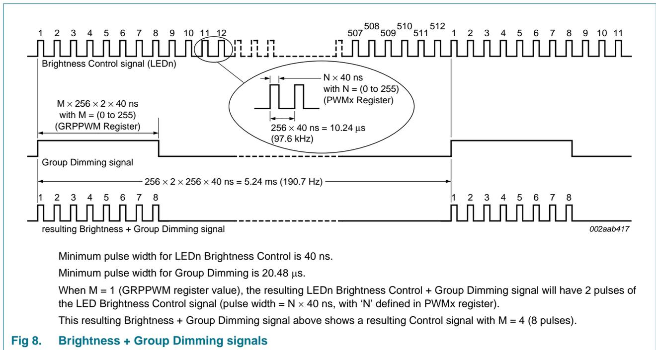
**Fig 8. Brightness + Group Dimming signals**
