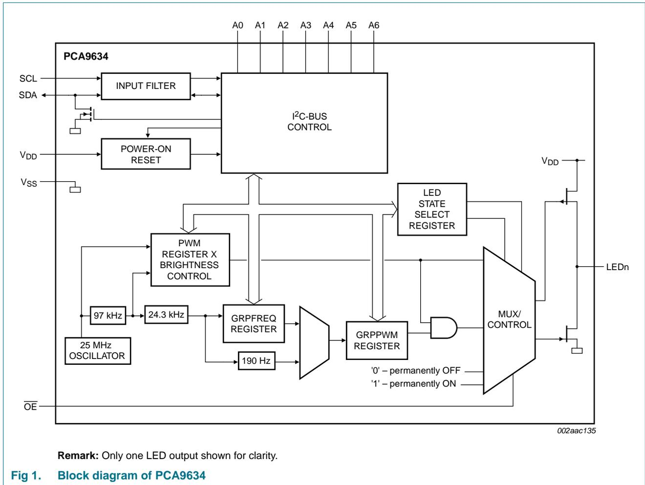
Fig 1. Block diagram of PCA9634
