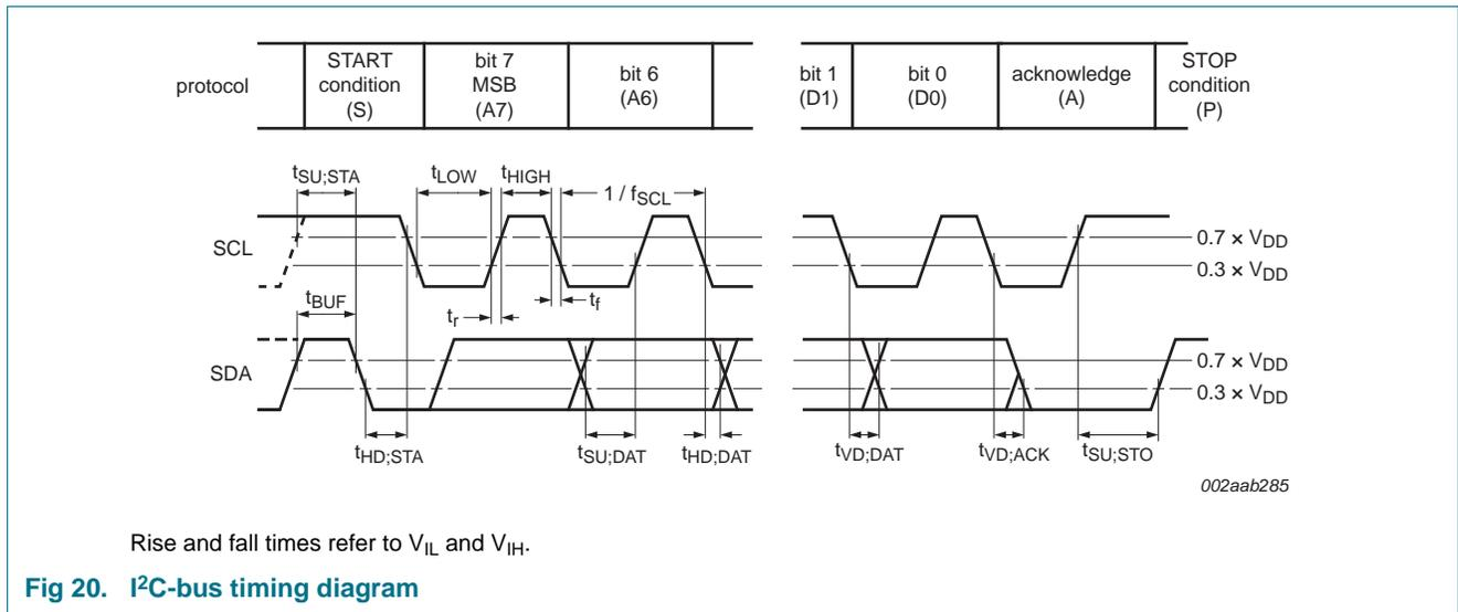
Fig 20. I<sup>2</sup>C-bus timing diagram
