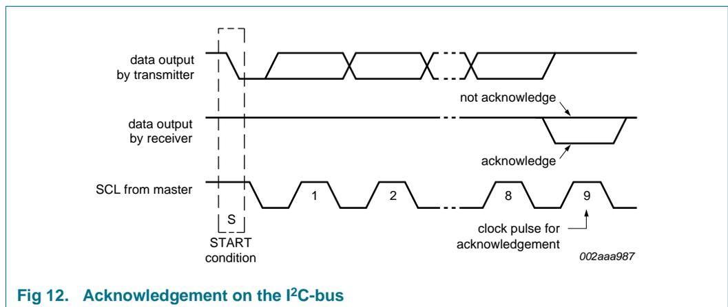
Fig 12. Acknowledgement on the I<sup>2</sup>C-bus
