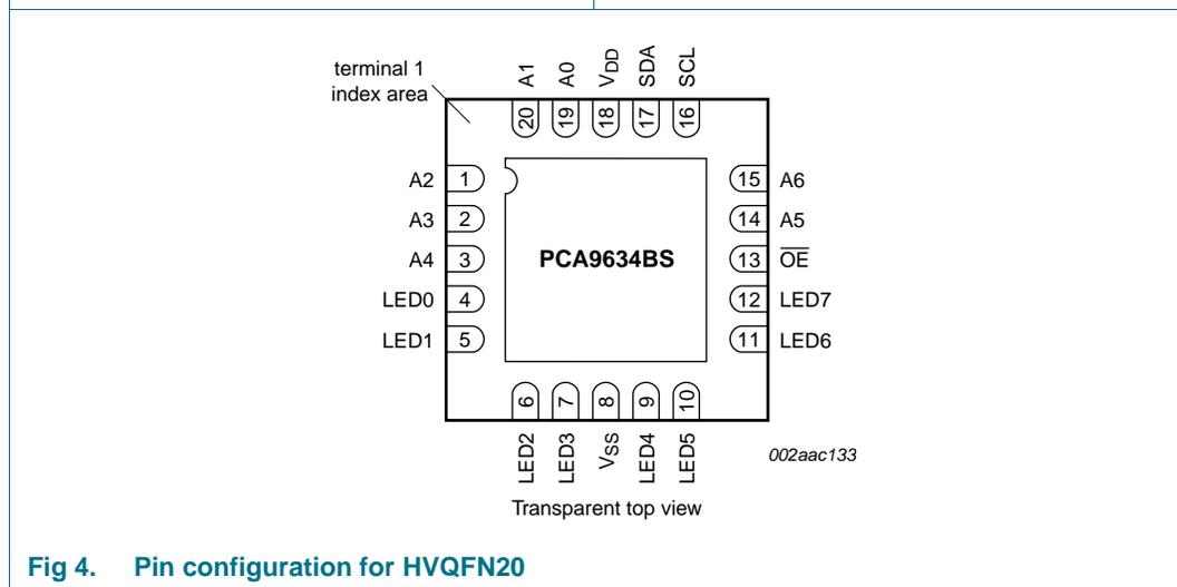
Fig 4. Pin configuration for HVQFN20
