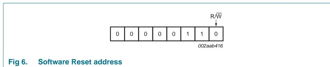
**Fig 6. Software Reset address**
