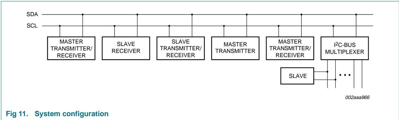
Fig 11. System configuration
