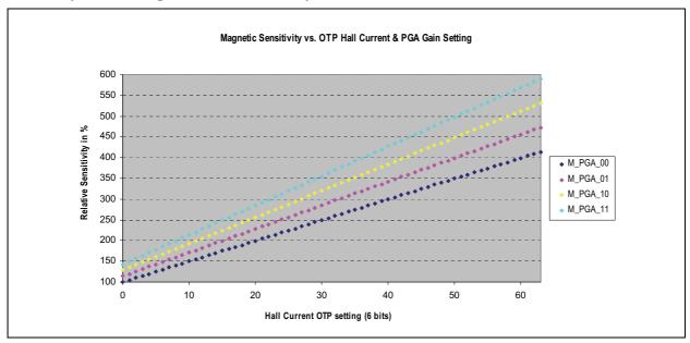
The amplitude of the output signal is programmable via sensitivity (6bit) and/or gain (2bit) settings (see Figure 25).
