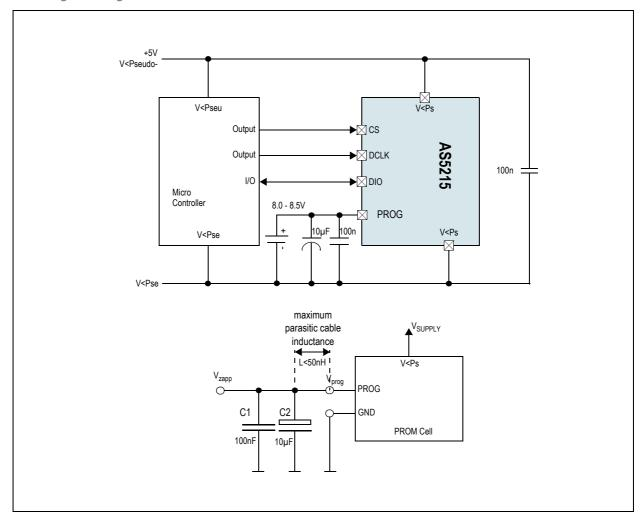
For programming of the OTP, an additional voltage has to be applied to the pin PROG. It has to be buffered by a fast 100nF capacitor (ceramic) and a  $10\mu F$  capacitor. The information to be programmed is set by command 25. The OTP bits 16 until 45 are used for ams OSRAM factory trimming and cannot be overwritten.
