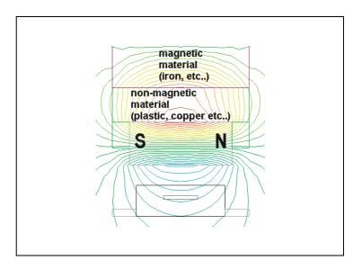
If the magnet has to be mounted inside a magnetic shaft, a possible solution is to place a non-magnetic spacer between shaft and magnet, as shown in Figure 20. While the magnetic field is rather distorted towards the shaft, there are still adequate field lines available towards the sensor IC. The distortion remains reasonably low.
