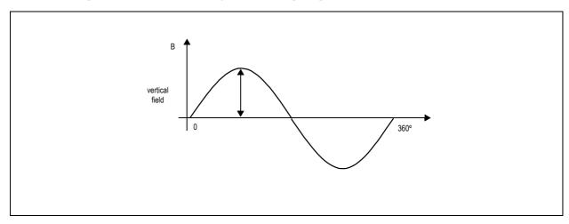
The recommended magnetic field, measured at the chip surface on a radius equal to the Hall sensor array radius (typ 1mm) should be within a certain range. This range lies between 45 and 75mT or between 20 and 80mT, depending on the encoder product.
