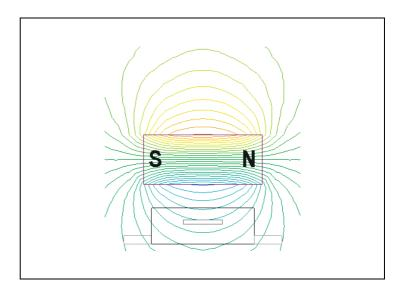
Figure 17 shows the ideal case with the magnet in air. No magnetic materials are anywhere nearby.
