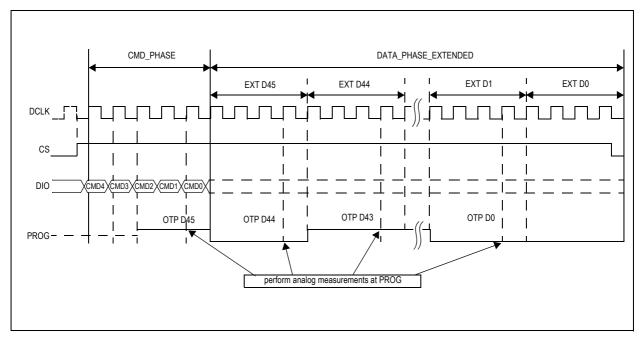
Figure 30: Serial Bit Sequence (16-Bit Read / Write)
