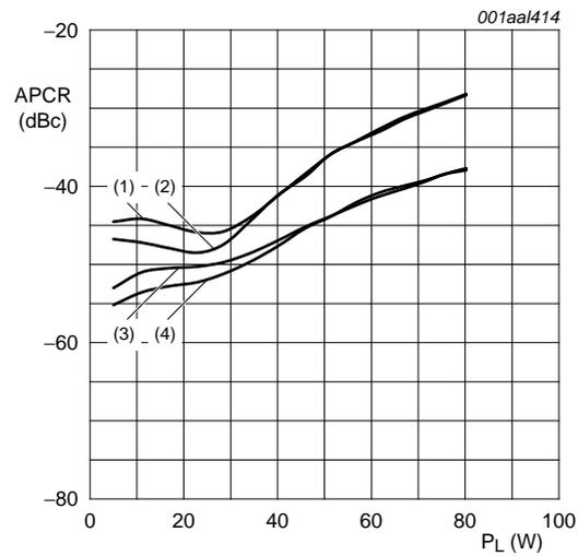
$V_{DS} = 28\text{ V}; I_{Dq} = 2000\text{ mA}$ .
