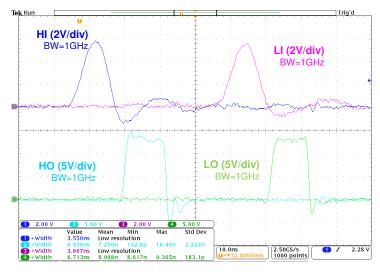
Figure 8-2. Input and Output Pulse Width
