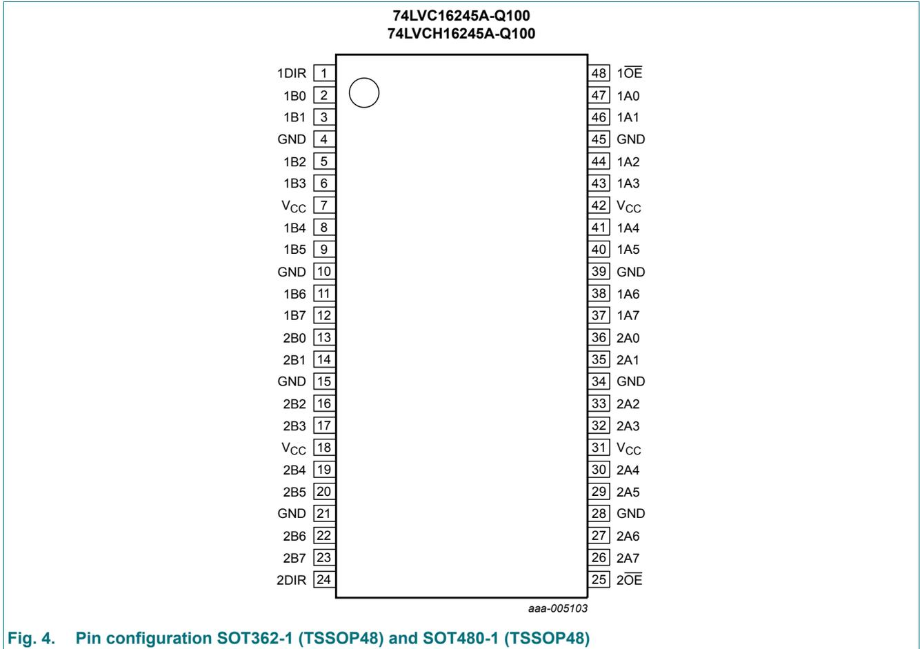
Fig. 4. Pin configuration SOT362-1 (TSSOP48) and SOT480-1 (TSSOP48)
