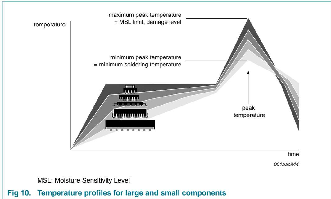
**Fig 10. Temperature profiles for large and small components**
