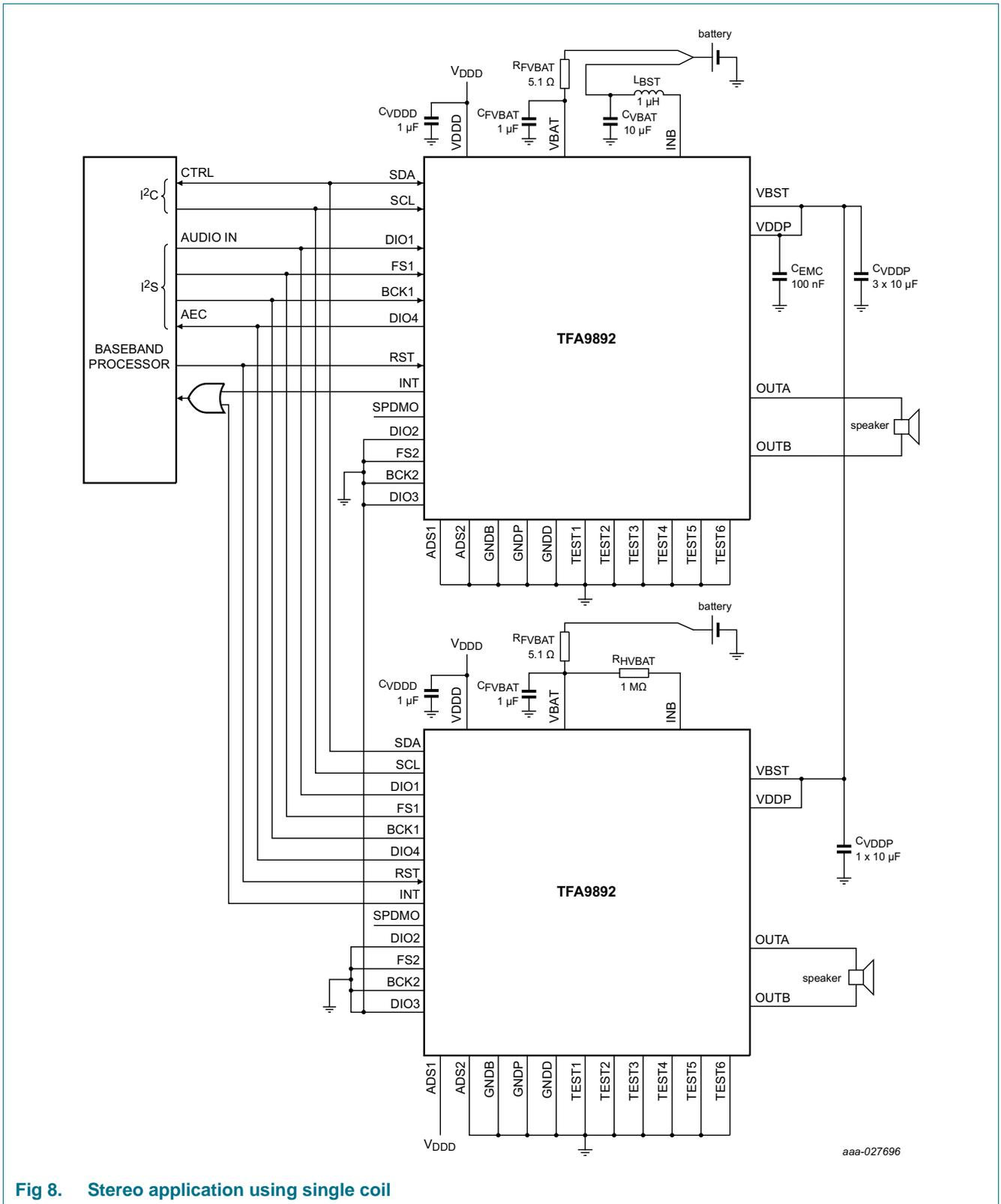
Fig 8. Stereo application using single coil
