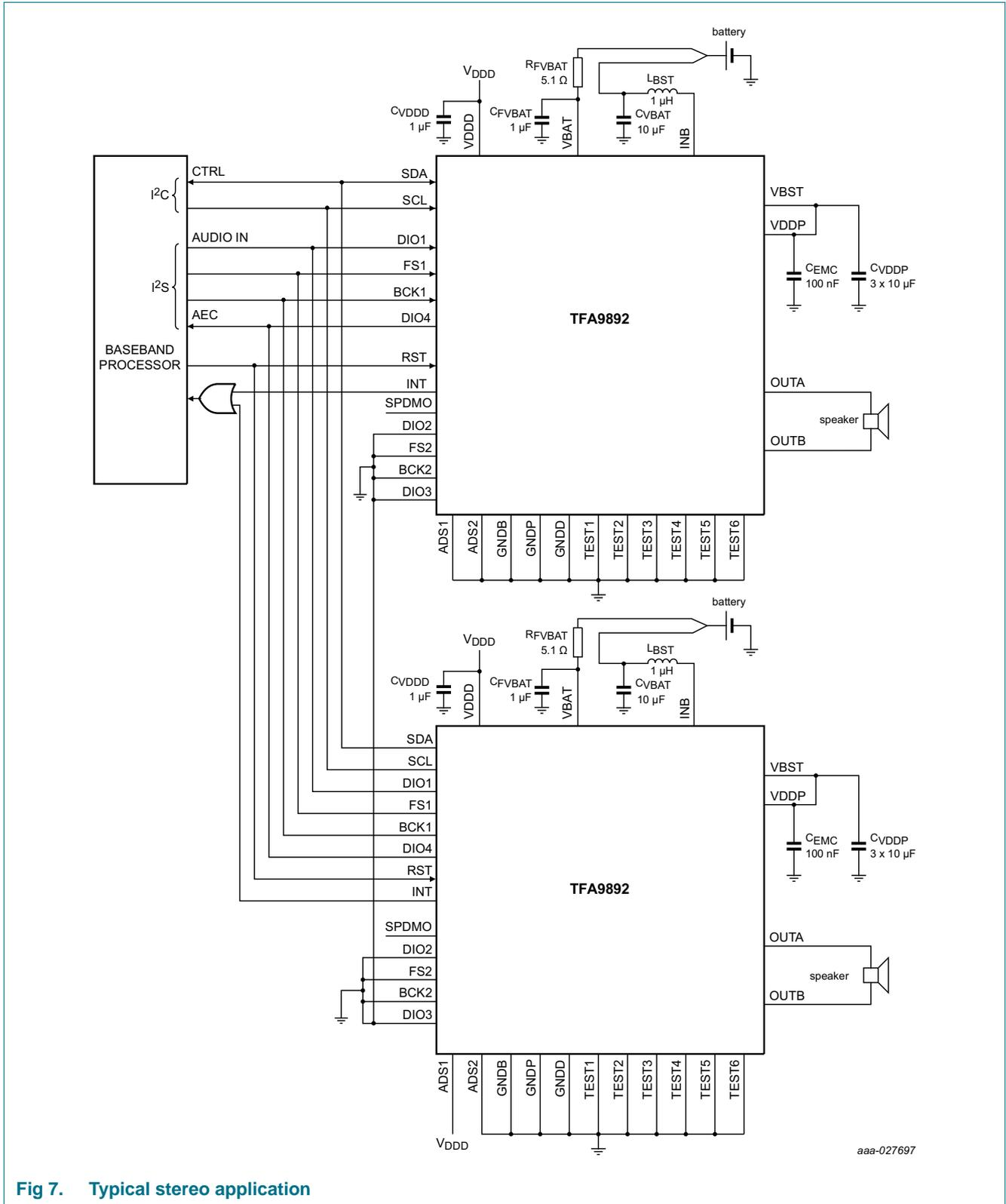
Fig 7. Typical stereo application
