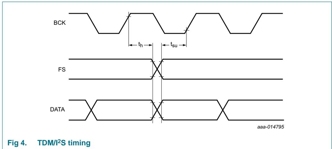
**Fig 4. TDM/I<sup>2</sup>S timing**
