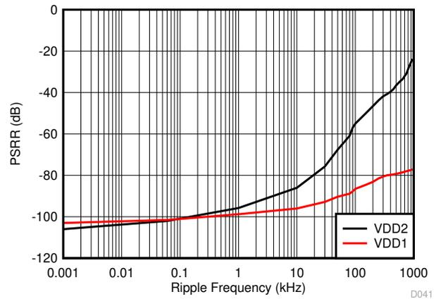
Figure 6-26. Power-Supply Rejection Ratio vs Ripple Frequency
