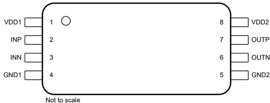
**Figure 5-1. DWL Package, 8-Pin SOIC (Top View)**
