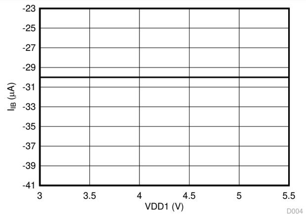
Figure 6-10. Input Bias Current vs High-Side Supply Voltage
