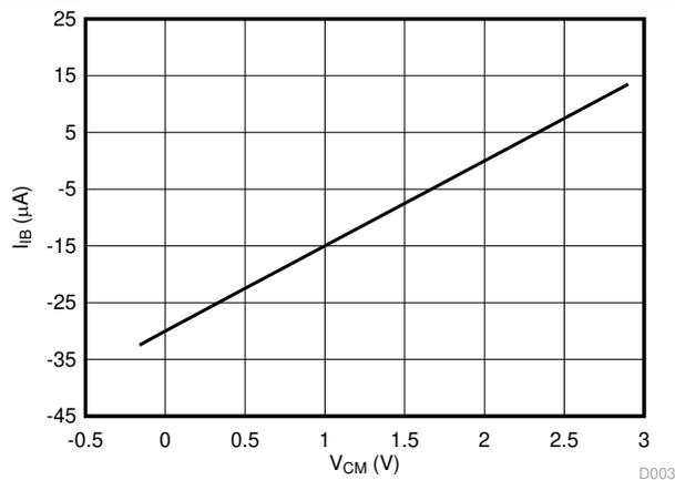
Figure 6-9. Input Bias Current vs Common-Mode Input Voltage
