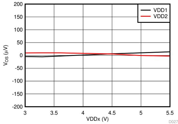
Figure 6-5. Input Offset Voltage vs Supply Voltage
