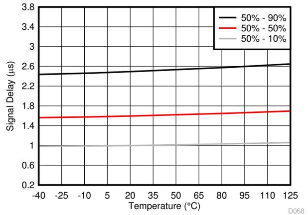
Figure 6-36.  $V_{IN}$  to  $V_{OUT}$  Signal Delay vs Temperature
