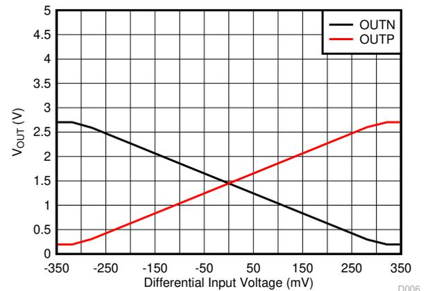
Figure 6-16. Output Voltage vs Input Voltage
