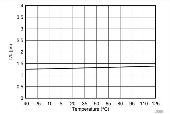
Figure 6-34. Output Rise and Fall Time vs Temperature
