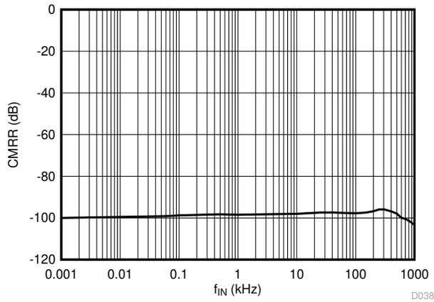
Figure 6-7. Common-Mode Rejection Ratio vs Input Frequency
