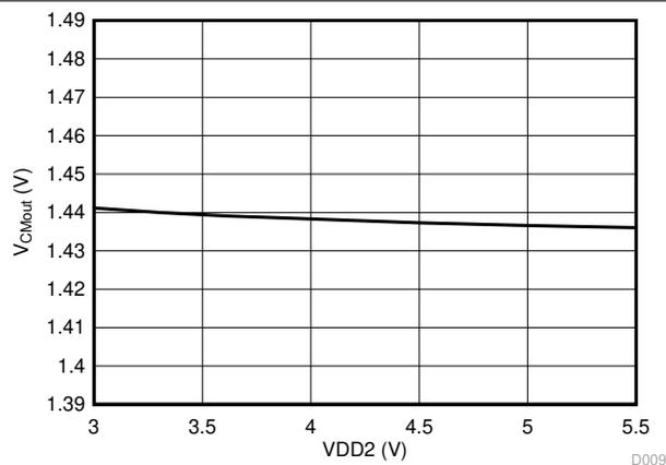
Figure 6-27. Output Common-Mode Voltage vs Low-Side Supply Voltage
