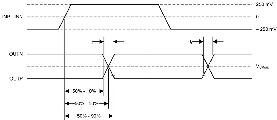
**Figure 6-1. Rise, Fall, and Delay Time Definition**
