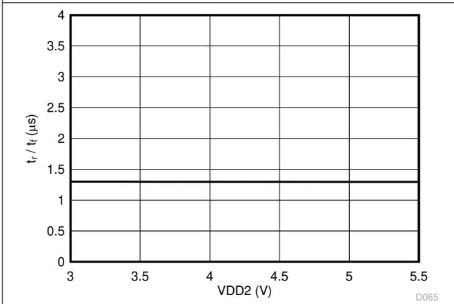
Figure 6-33. Output Rise and Fall Time vs Low-Side Supply
