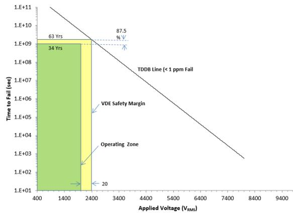
$T_A$  up to 150°C, stress-voltage frequency = 60 Hz, isolation working voltage = 2000  $V_{RMS}$ , operating lifetime = 34 year
