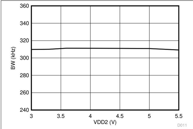
Figure 6-29. Output Bandwidth vs Low-Side Supply Voltage
