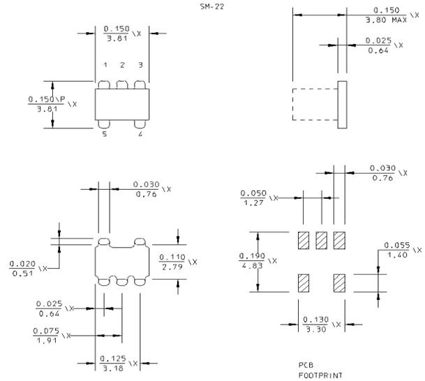
Dimensions are inches (millimeters)  $\pm 0.015$  (0.38) unless otherwise specified.
