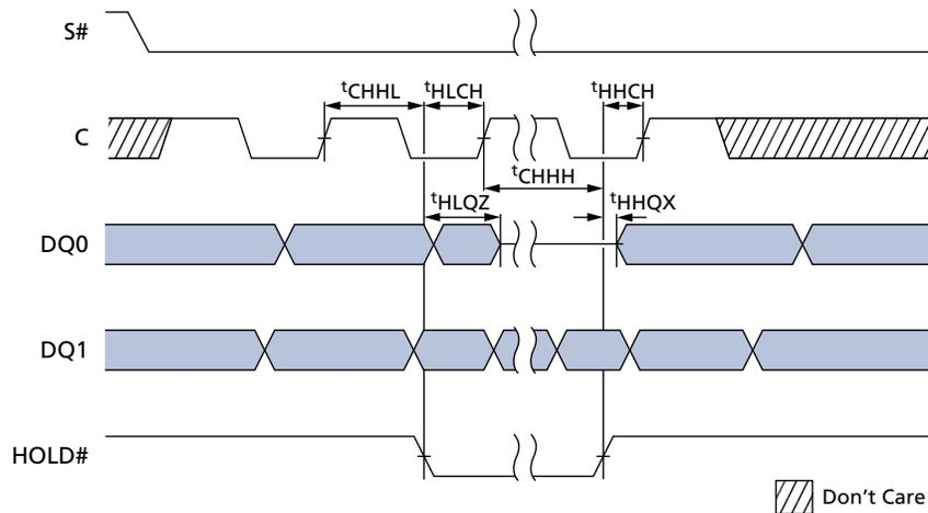
**Figure 47: Output Timing for STR**
