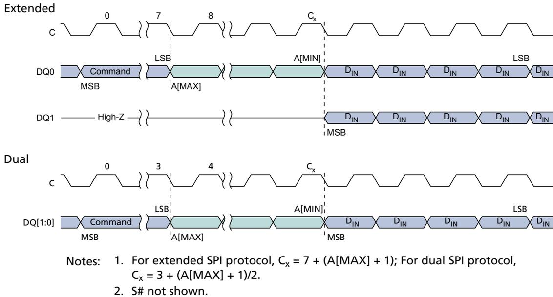
**Figure 29: EXTENDED DUAL INPUT FAST PROGRAM Command**
