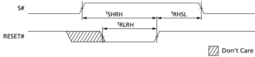
Figure 42: Reset Enable and Reset Memory Timing
