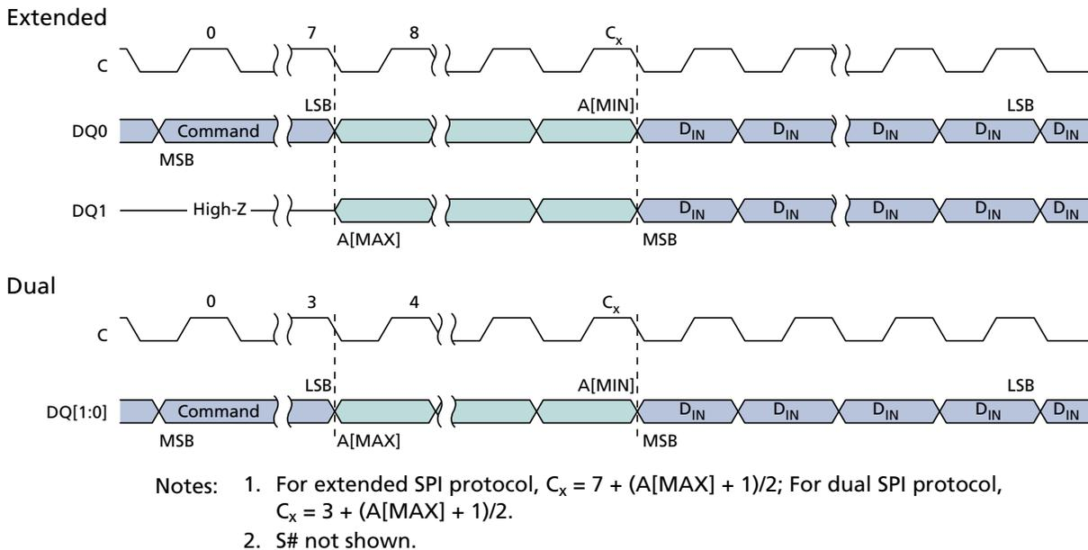
Figure 30: QUAD INPUT FAST PROGRAM Command
