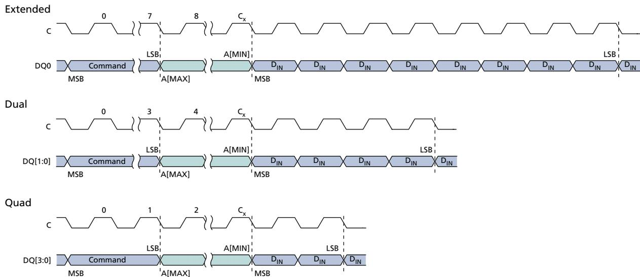
Note: 1. For extended SPI protocol,  $C_x = 7 + (A[\text{MAX}] + 1)$ ; For dual SPI protocol,  $C_x = 3 + (A[\text{MAX}] + 1)/2$ ; For quad SPI protocol,  $C_x = 1 + (A[\text{MAX}] + 1)/4$ .
