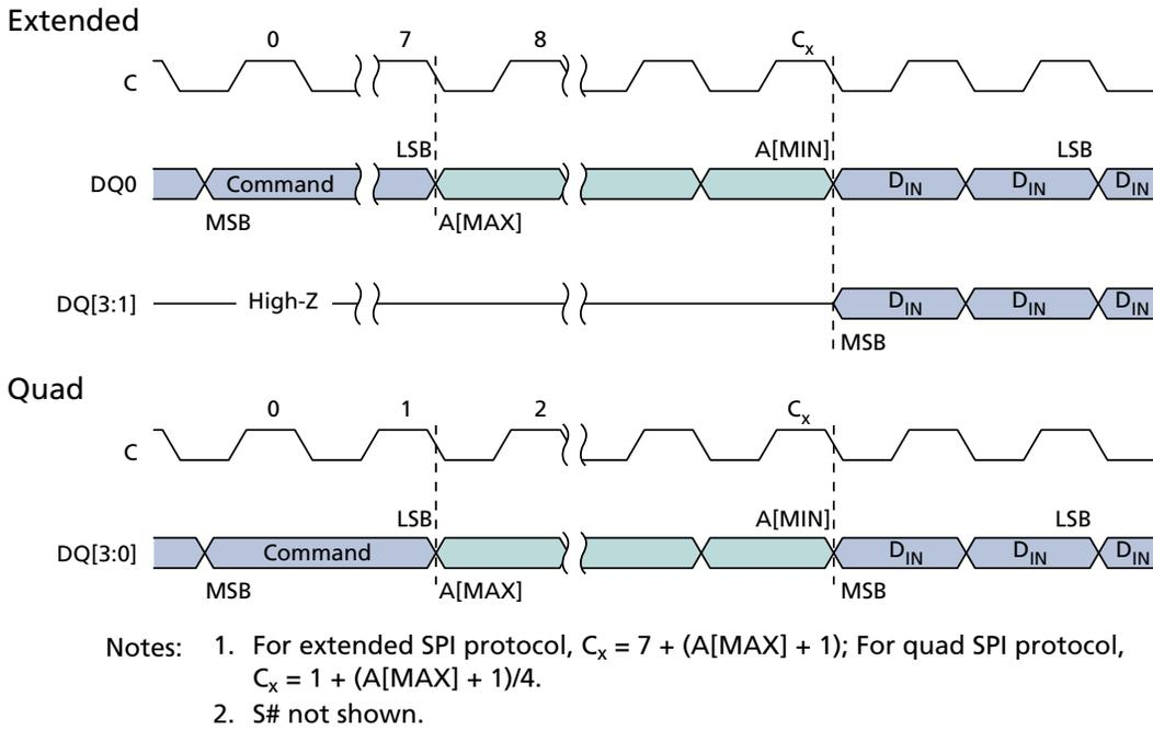
Figure 31: EXTENDED QUAD INPUT FAST PROGRAM Command
