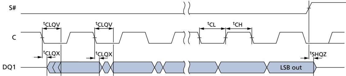
**Figure 48: Output Timing for DTR**
