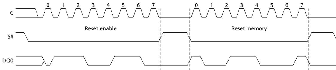
Figure 43: Serial Input Timing STR
