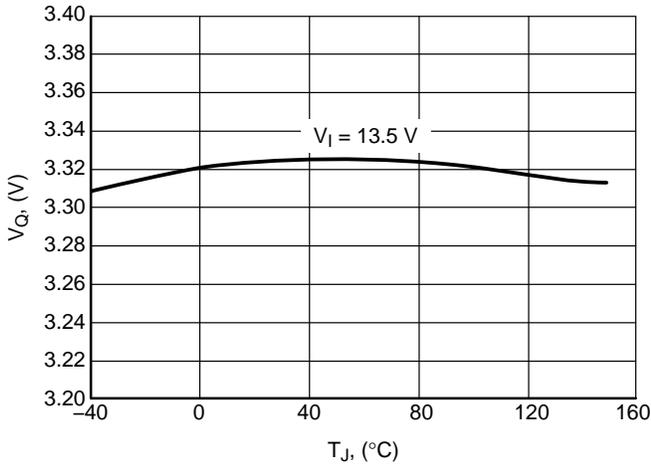
Figure 25. Output Voltage  $V_Q$  vs. Temperature  $T_J$
