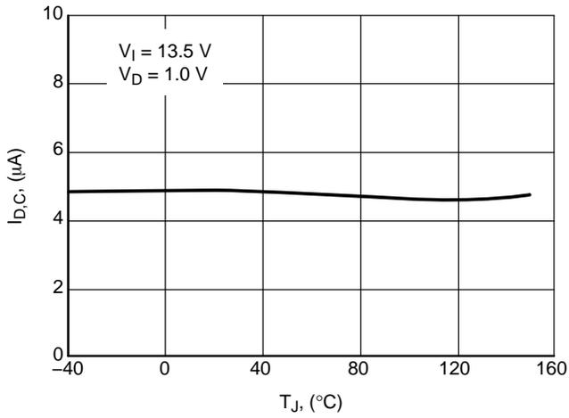
Figure 19. Charge Current  $I_{D,C}$  vs. Temperature  $T_J$
