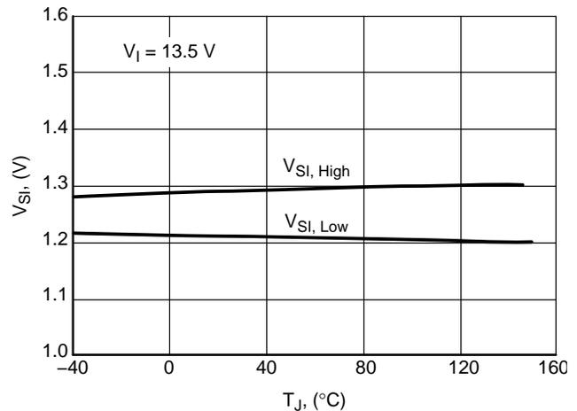
Figure 24. Sense Threshold  $V_{S1}$  vs. Temperature  $T_J$
