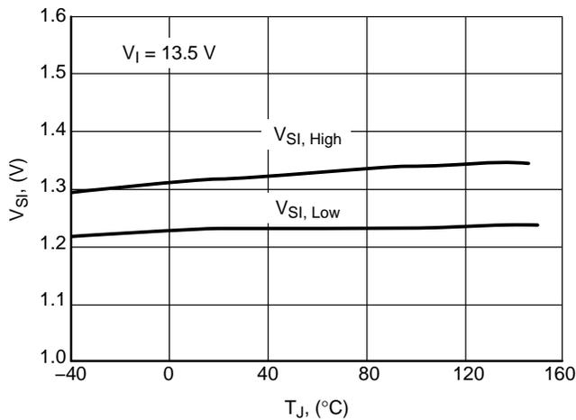
Figure 11. Sense Threshold  $V_{Si}$  vs. Temperature  $T_J$
