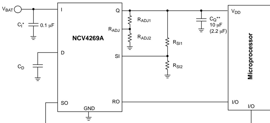
\* $C_1$  required if regulator is located far from the power supply filter.
