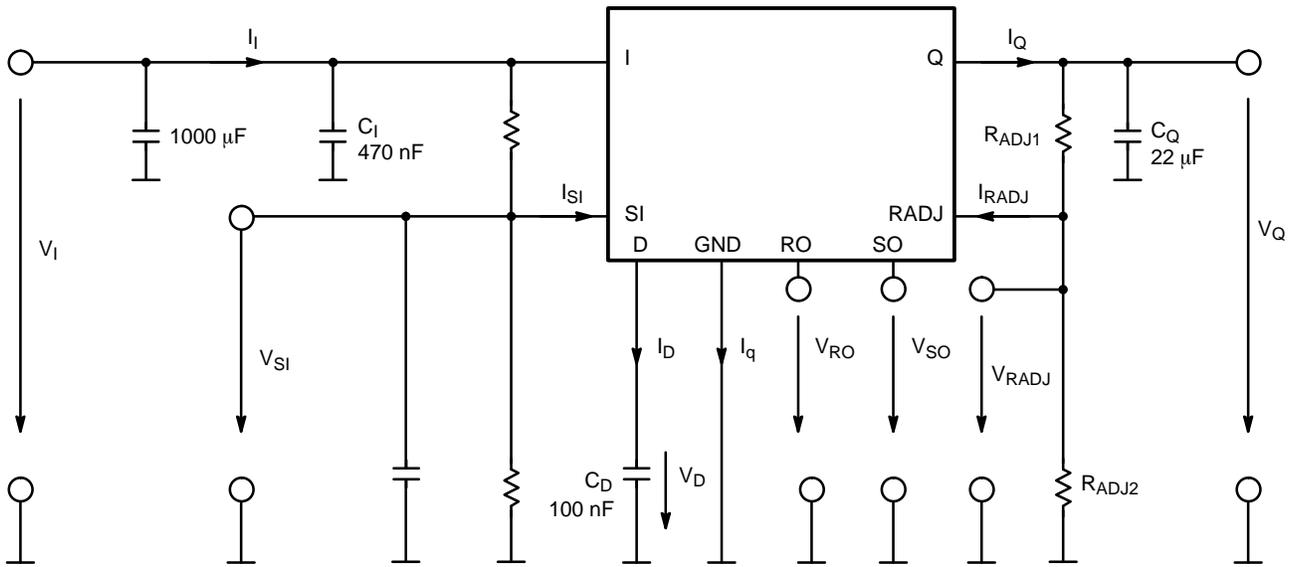
Figure 2. Measuring Circuit
