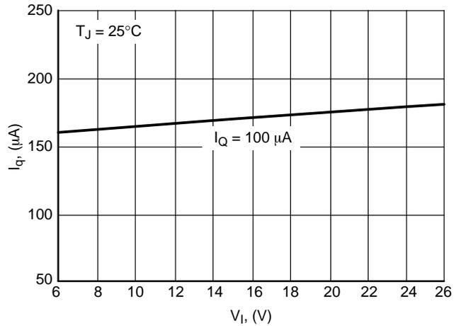
Figure 30. Quiescent Current  $I_q$  vs. Input Voltage  $V_I$
