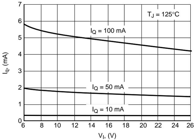
Figure 29. Quiescent Current  $I_q$  vs. Input Voltage  $V_I$
