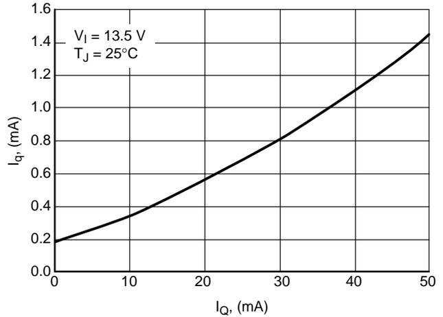
Figure 28. Current Consumption  $I_q$  vs. Output Current  $I_Q$
