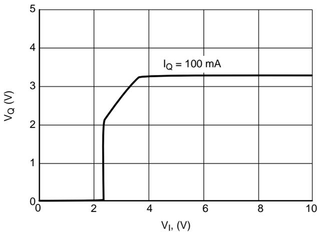
Figure 23. Output Voltage  $V_Q$  vs. Input Voltage  $V_I$
