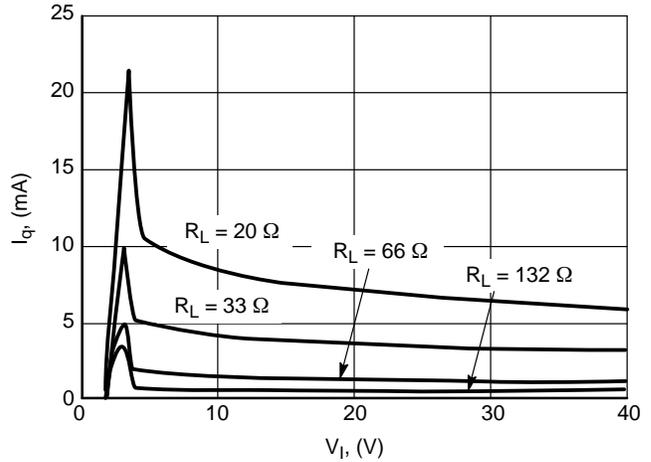
Figure 22. Current Consumption  $I_q$  vs. Input Voltage  $V_I$
