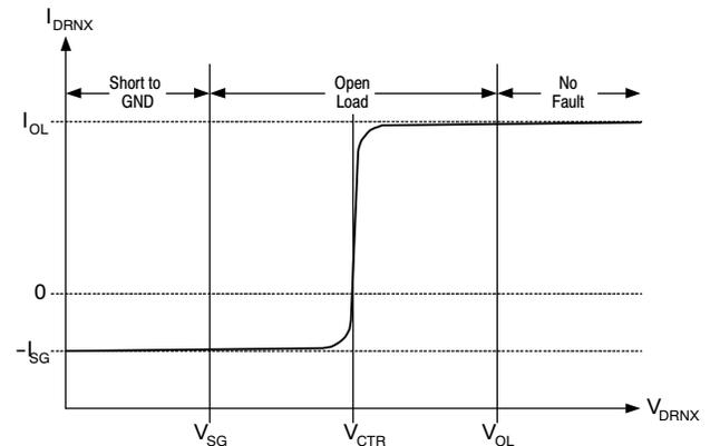
Figure 14.  $DRN_X$  Bias and Fault Detection Zones
