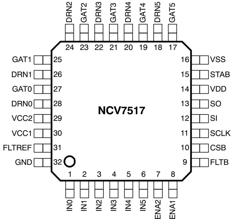
Figure 3. 32 Pin LQFP Pinout (Top View)
