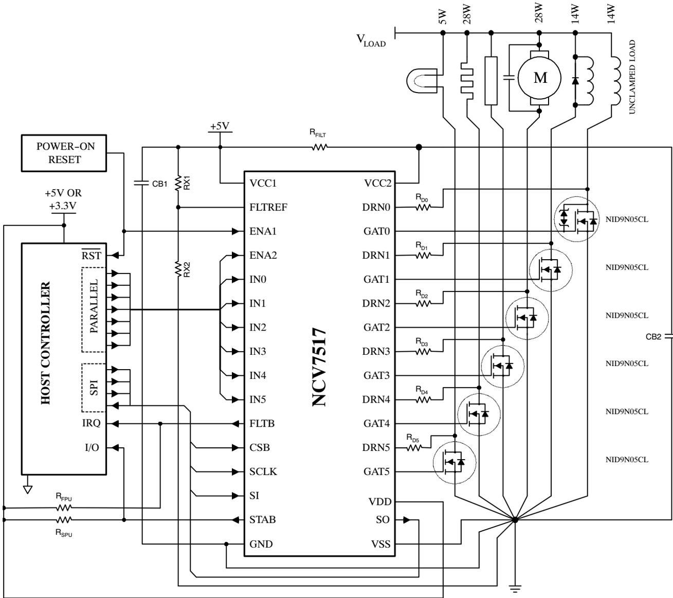
Figure 2. Application Diagram
