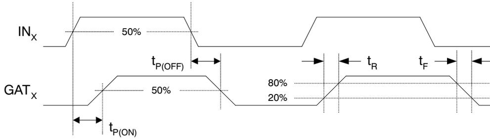
Figure 4. Gate Driver Timing Diagram – Parallel Input
