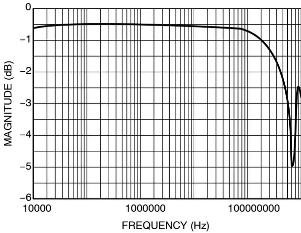
**Figure 4. Typical Bandwidth @  $V_{CC} = 5.5$  V, 25°C**
