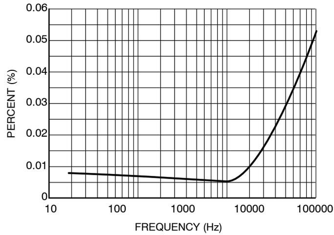
**Figure 6. Typical Total Harmonic Distortion @  $V_{CC} = 4.5$  V**
