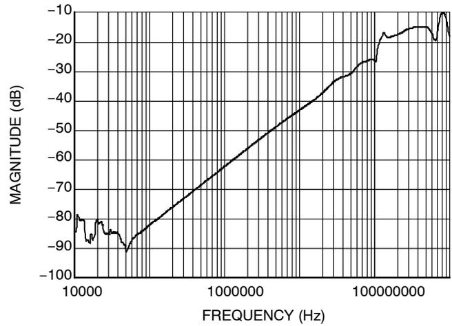
**Figure 5. Off-Channel Isolation @  $V_{CC} = 5.5$  V, 25°C**
