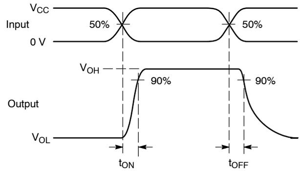
Figure 1.  $t_{ON}/t_{OFF}$
