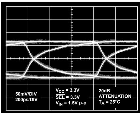
Figure 22. Eye Pattern; 1.5 Gbps,  $V_{CC} = 3.3V$ , PRBS 31
