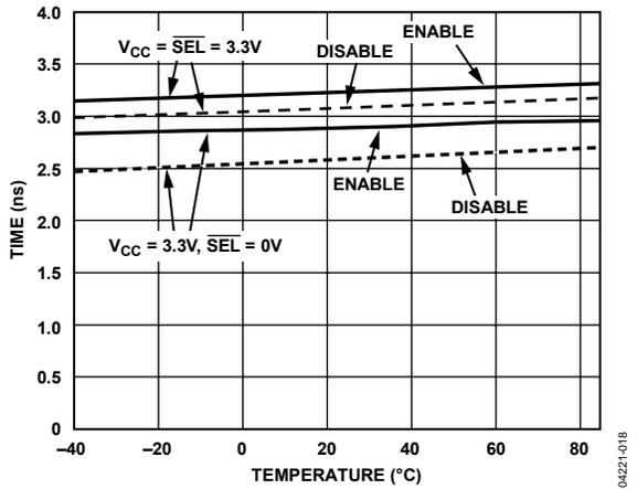
Figure 18. Enable/Disable Time vs. Temperature
