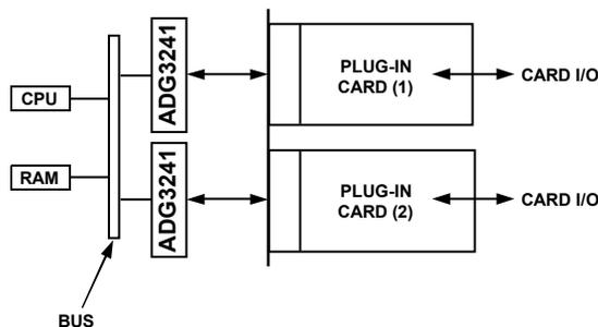
Figure 35. ADG3241 in a Hot Plug Application
