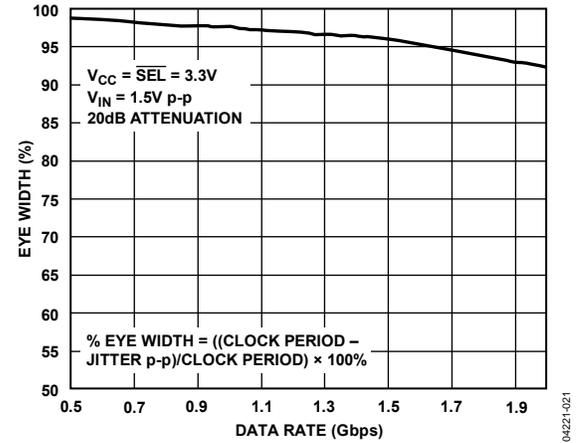
Figure 21. Eye Width vs. Data Rate; PRBS 31
