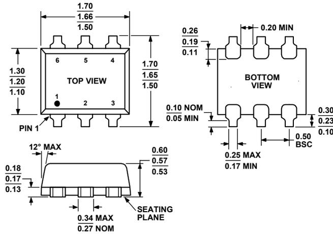
Figure 37. 6-Lead Small Outline Transistor Package [SOT-66] (RY-6-1)
