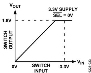
Figure 33. 3.3 V to 1.8 V Voltage Translation,  $\overline{SEL} = 0 V$
