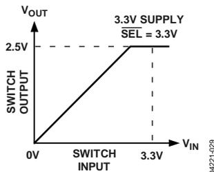
Figure 29. 3.3 V to 2.5 V Voltage Translation,  $\overline{SEL} = V_{CC}$
