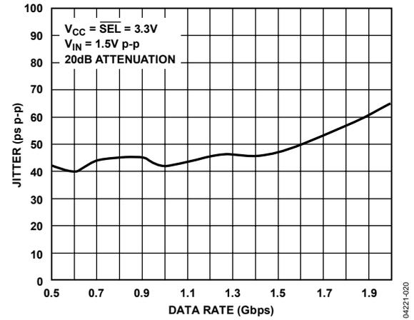
Figure 20. Jitter vs. Data Rate; PRBS 31
