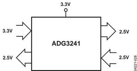
Figure 28. 3.3 V to 2.5 V Voltage Translation,  $\overline{SEL} = V_{CC}$
