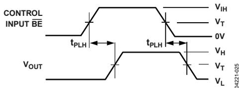
Figure 25. Propagation Delay
