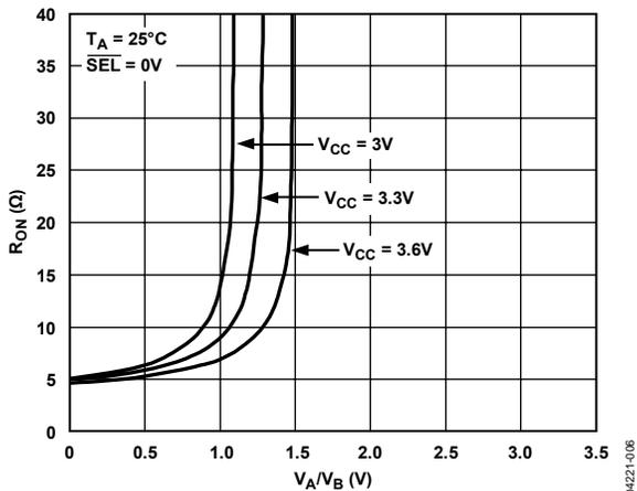
Figure 6. On Resistance vs. Input Voltage
