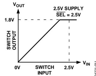
Figure 31. 2.5 V to 1.8 V Voltage Translation,  $\overline{SEL} = V_{CC}$
