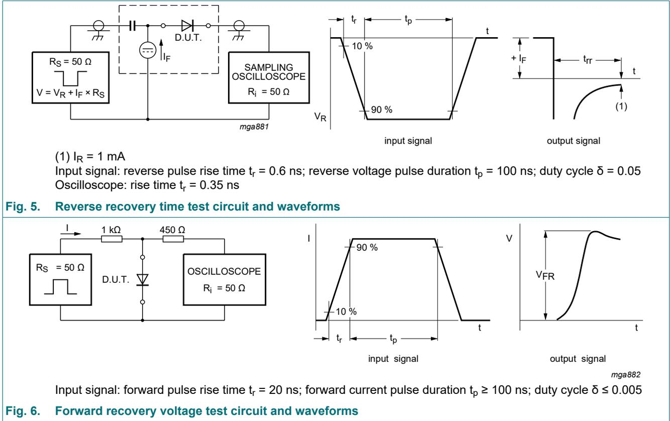
Fig. 5. Reverse recovery time test circuit and waveforms
