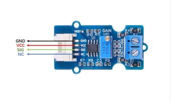
Grove AC Voltage Sensor is perfect for measuring RMS AC voltages for accurate DIY energy meters. It has adjustable gain for different voltage inputs (120V-240V AC), and it supports a 5 - 3.3v DC power supply.
