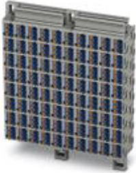
Marshalling patchboard, Nom. voltage: 500 V, Nominal current: 17.5 A, Cross section: 0.14 mm<sup>2</sup> - 2.5 mm<sup>2</sup>, AWG: 12 - 26, Connection type: Push-in connection, Number of positions: 80, Number of connections: 480, Width: 110 mm, Length: 102 mm, Color: gray, Color of connection elements: blue, Assembly: Wall mounting
