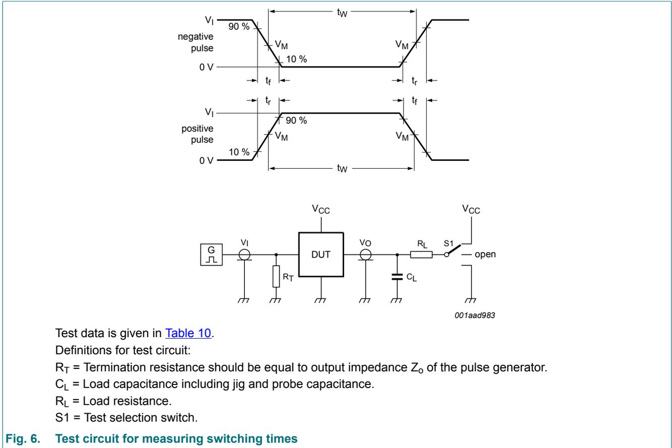
Fig. 6. Test circuit for measuring switching times
