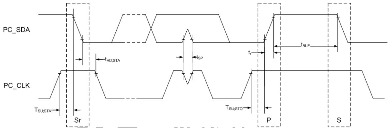
Figure 2. I<sup>2</sup>C Mode Timing
