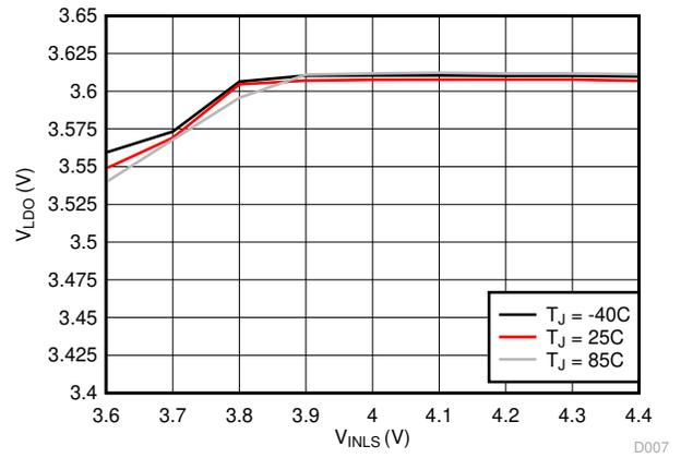
Figure 8-12. LDO Line Regulation (VLDO = 3.6 V)
