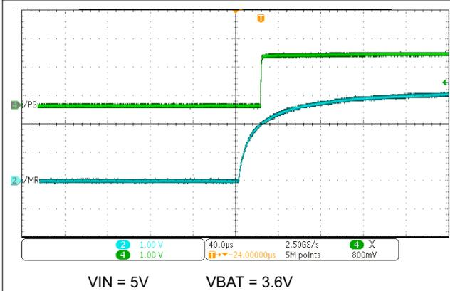
**Figure 10-12.  $\overline{\text{PG}}$   $\overline{\text{MR}}$  Level Shift Function -  $\overline{\text{MR}}$  Rising**
