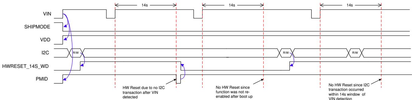
**Figure 9-7. 14-Second Watchdog for HW Reset Behavior**
