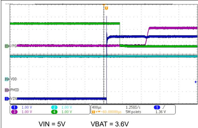
**Figure 10-10.  $\overline{\text{PG}}$  Power Good Function - IN Supply Insertion**
