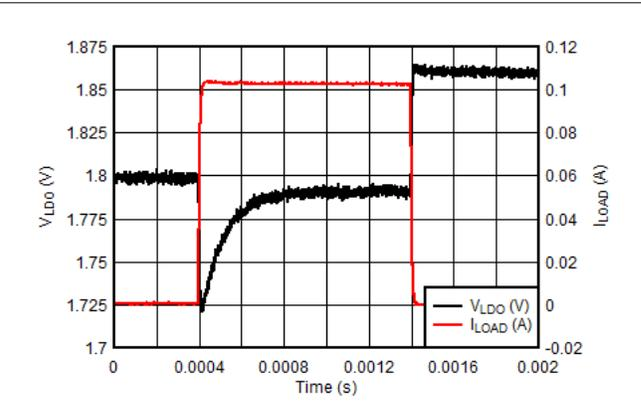
**Figure 10-17. LDO Load Transient - VLDO = 1.8V**
