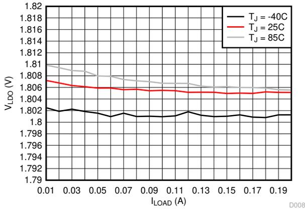
Figure 8-7. LDO Load Regulation (VLDO = 1.8 V)
