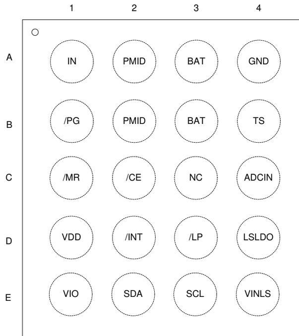
**Figure 7-1. YFP Package 20-Pin DSBGA Top View**
