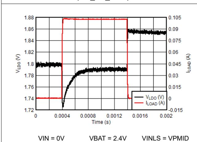
**Figure 10-18. LDO Load Transient - VLDO = 1.8V**
