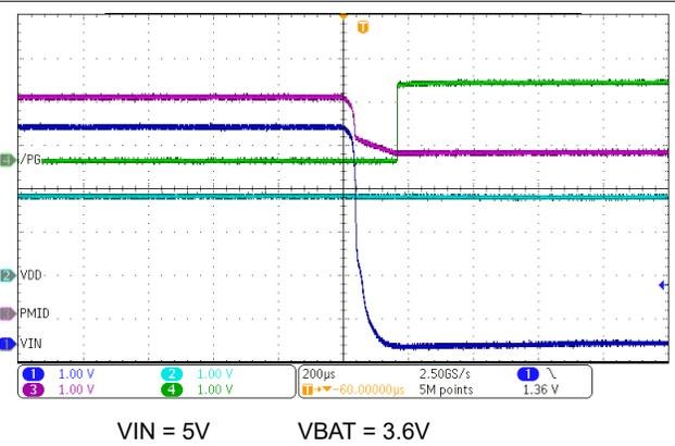
**Figure 10-11.  $\overline{\text{PG}}$  Power Good Function - IN Supply Removal**
