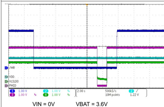
**Figure 10-6. HW Reset on  $\overline{MR}$  Long Button Press**
