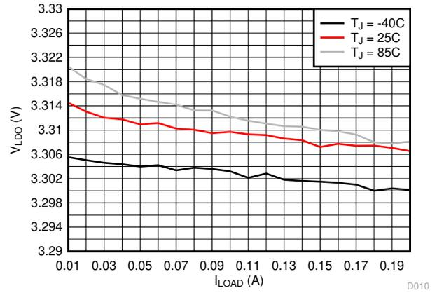
Figure 8-8. LDO Load Regulation (VLDO = 3.3 V)
