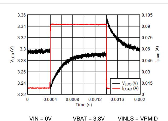
**Figure 10-19. LDO Load Transient - VLDO = 3.3V**
