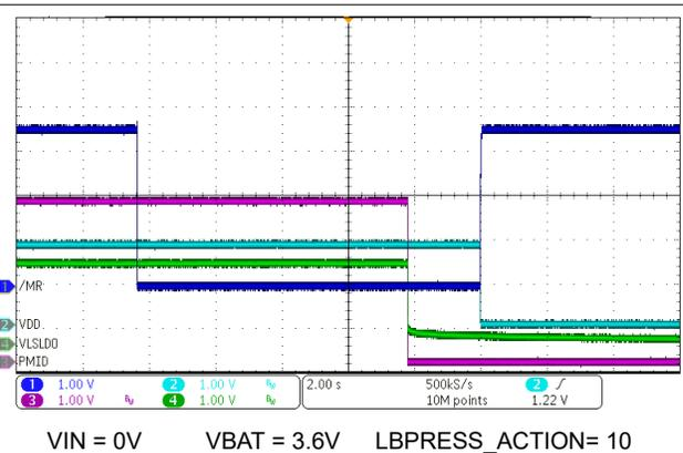
**Figure 10-7. Ship Mode Entry with  $\overline{MR}$  Long Button Press**
