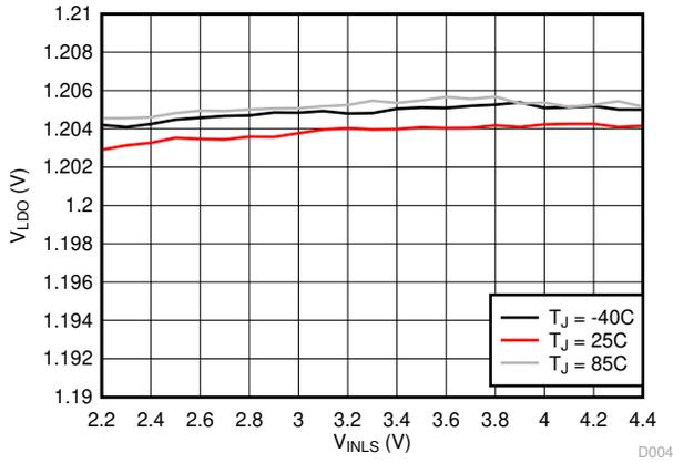
Figure 8-9. LDO Line Regulation (VLDO = 1.2 V)
