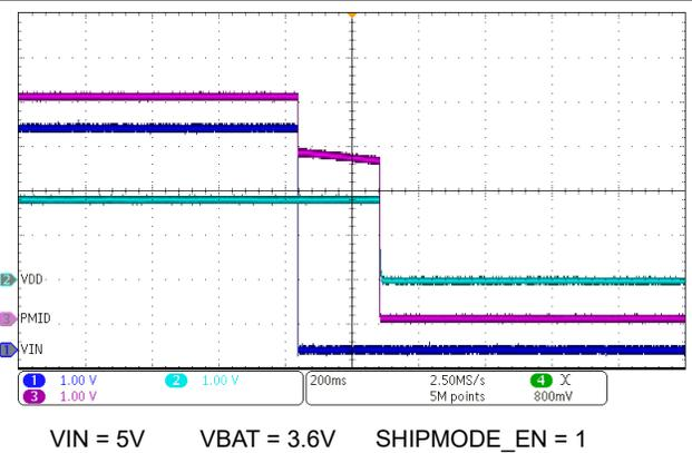
**Figure 10-9. Ship Mode Entry on IN Supply Removal**
