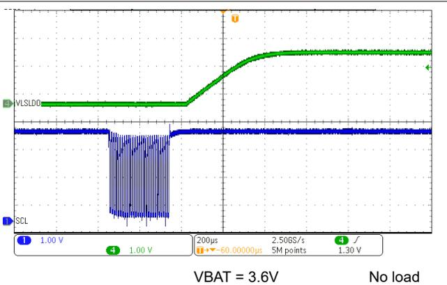
**Figure 10-15. LDO Enable Through I<sup>2</sup>C (EN\_LS\_LDO)**
