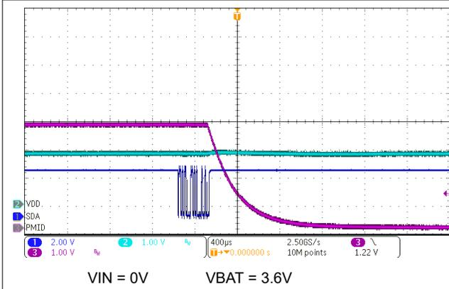
**Figure 10-8. HW Reset Through I<sup>2</sup>C Command**
