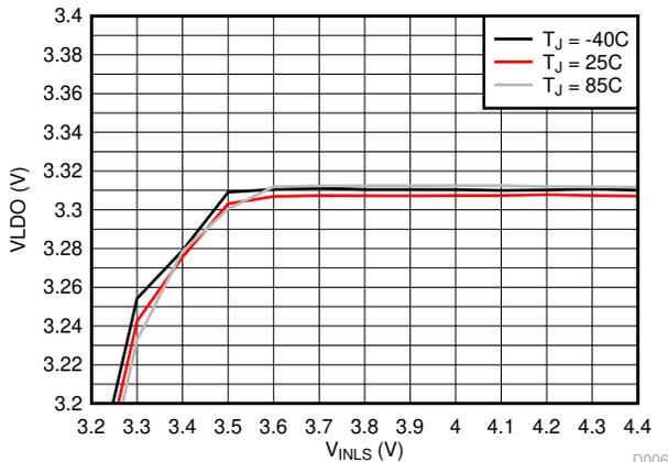
Figure 8-11. LDO Line Regulation (VLDO = 3.3 V)
