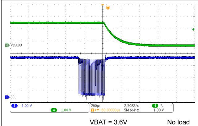
**Figure 10-16. LDO Disable Through I<sup>2</sup>C (EN\_LS\_LDO)**
