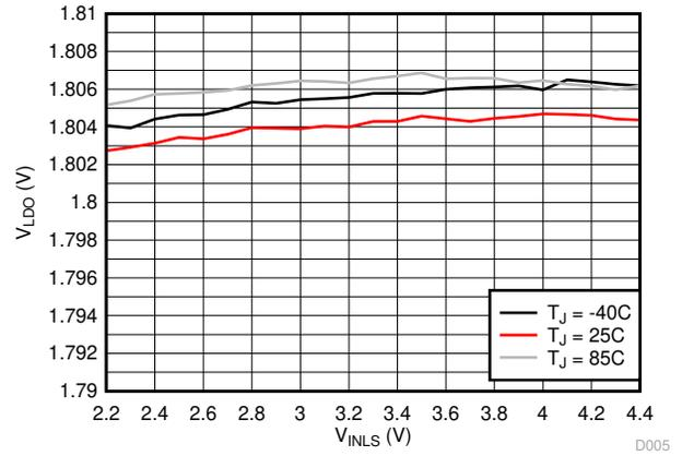
Figure 8-10. LDO Line Regulation (VLDO = 1.8 V)
