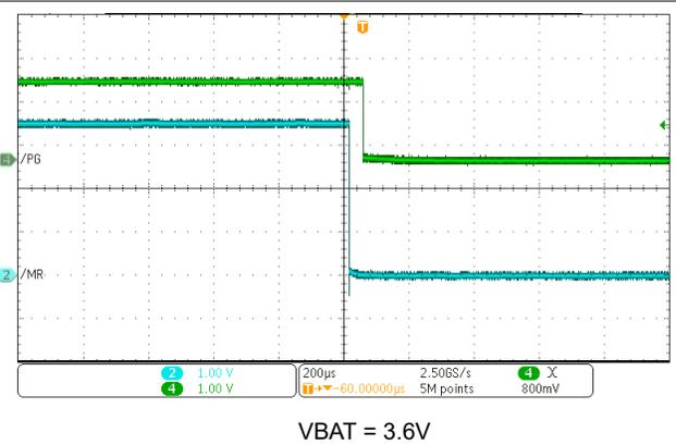
**Figure 10-13.  $\overline{\text{PG}}$   $\overline{\text{MR}}$  Level Shift Function -  $\overline{\text{MR}}$  Falling**
