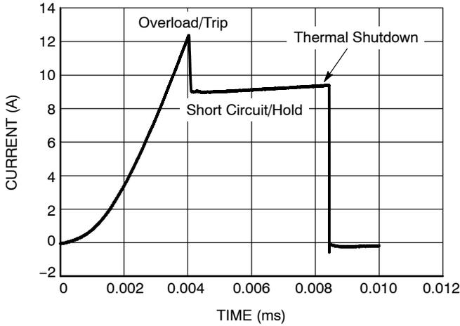
Figure 6. Slow Fault Current Limit Characteristic of NIS5020
