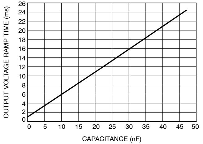
Figure 9. Output Voltage Ramp Time vs.  $dv/dt$  Capacitance
