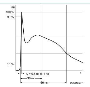
Fig. 3. ESD pulse waveform according to IEC 61000-4-2
