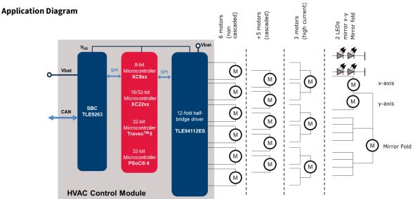
**Example:** The TLE94112ES, 12-fold half-bridge, is designed to either drive 6 DC motors up to 0.9A in parallel mode or 11 DC motors up to 0.9A in cascaded mode or up to 3 DC motors up to 1.8A by paralleling two outputs each. The device is sold in a TSDSO-24 package and is pin and function compatible with the 6-, 8-, and 10-fold half-bridge of the TLE94xyz family.
