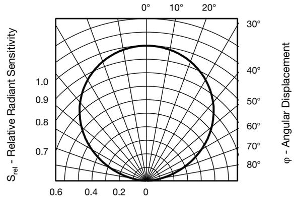
Fig. 7 - Relative Radiant Sensitivity vs. Angular Displacement
