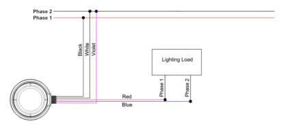
Wiring Diagram C - 208/240VAC & 480VAC Line voltage wiring diagram.
