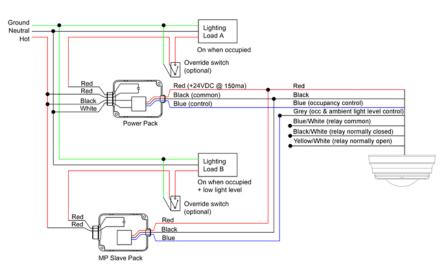
Wiring Diagram D - Low voltage sensor wiring diagram.
