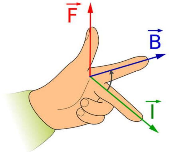
The direction of the force shows the direction that the motor coil will move, and hence the direction of rotation.
