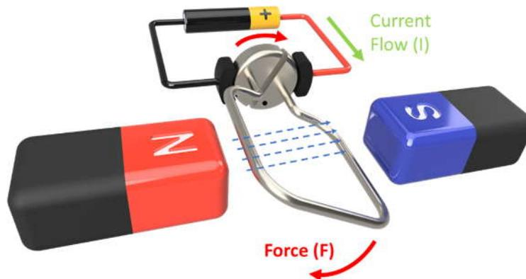
As the coil rotates towards the opposite side the force would change direction, and the motor would not spin.
