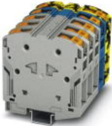
High-current terminal block, Blocked, Connection method: Power-Turn connection, Cross section: 10 mm<sup>2</sup> - 70 mm<sup>2</sup>, AWG: 8 - 2/0, Width: 80 mm, Color: gray/blue, Mounting type: NS 35/15
