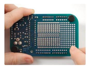
Finally, you can finish your kit by placing the four rubber bumpers over the mounting hole spots. These will keep the Menta off your desk to avoid scratching it, or accidentally shorting against a piece of wire.
