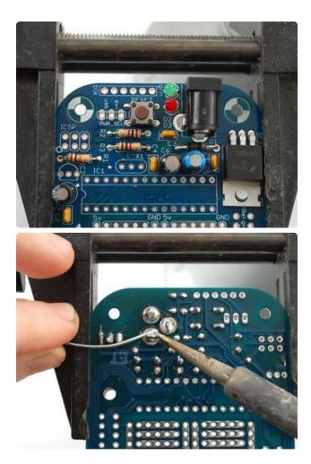
Now we can place the big power jack. This is how we can plug in a battery or power adapter.
