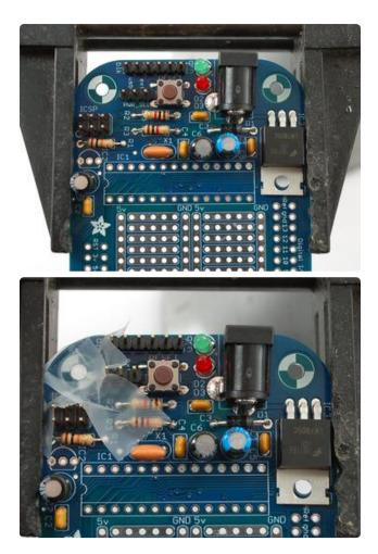
Place one piece of the header, the 6-pin piece, into the spot right next to the green LED. Make sure the short legs are sticking down into the PCB and the long legs are sticking up. This is the programming header. This is where you can connect an FTDI cable or FTDI friend to reprogram the Menta.
