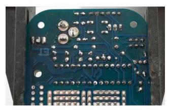
Solder in all 28 pins of the socket and the 3.3V regulator.
