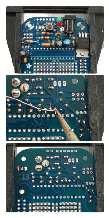
Next up is the 16.00 MHz crystal X1. This crystal is what lets the Menta chip run at a brisk 16 million clocks per second. This oscillator comes in a orange shape with three pins. Luckily, it's symmetric so just place it any way you like.
