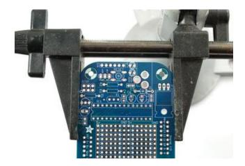
Place the circuit board in a vise so that you can easily work on it.
