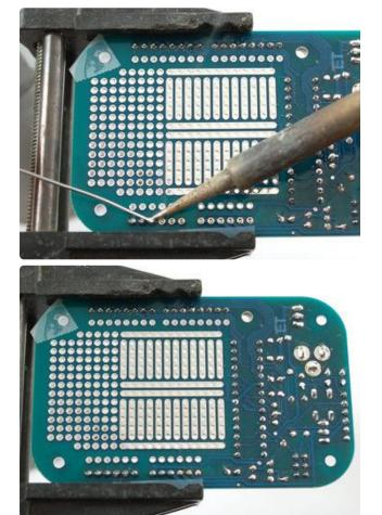
Solder in the 4 sets of header, all of the pins!
