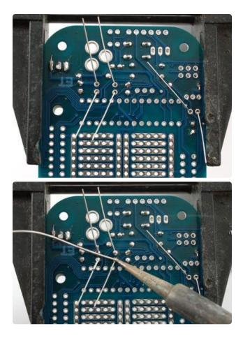
After you've triple-checked the polarity of the capacitors, flip over the PCB and solder them in.
