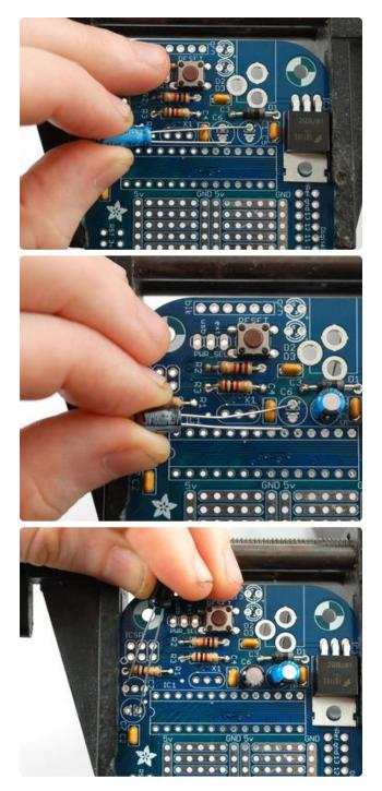
Next we will place the polarized electrolytic capacitors. These are the beefy versions of the ceramic capacitors we already placed. Ceramics are good for high frequency noise, and the electrolytics are good for low frequency noise, that's why we team them up together to cover all frequencies.
