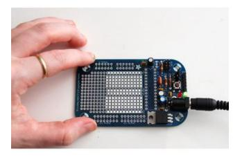
Now we can do a test, find a DC power adapter, 7VDC or higher, with a 2.1mm jack and center-polarity (these are nearly standard) and plug it in. With the jumper in place, you should see the Green LED light up. If not, something is wrong - either the LED is in backwards or your power supply isn't working. Go back and check your work until you can figure out what happened.
