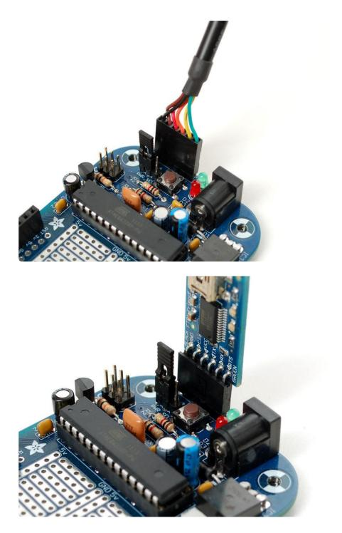
Connect the FTDI adapter to your computer and start the IDE. Select the COM or / dev/tty port that is created when you plugged in the FTDI adapter.
