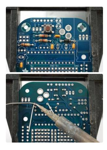
Now we will place our first non-symmetric component, a diode! The diode only conducts current in one direction. We use this diode for protecting the Menta - since it can only work in one direction it makes sure we don't connect negative voltages into the DC plug that could damage or destroy the electronics. This particular diode is a 1N4001 model, which is extremely common power diode that can handle over an Amp of current.
