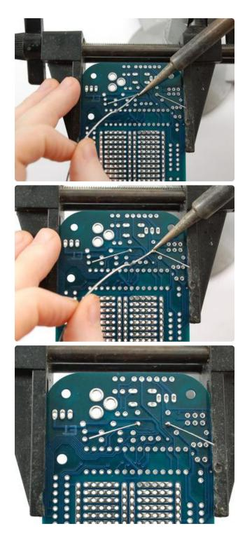
Now we will solder in the first part. Heat up your soldering iron (about 700 degrees F is common but you may need to adjust it higher for lead-free).
