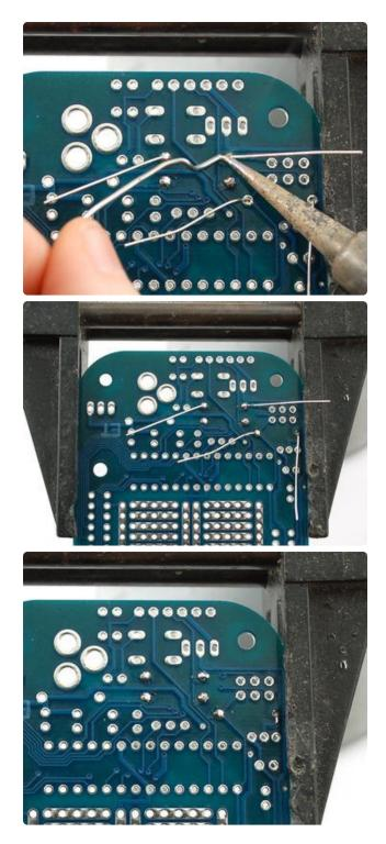
Flip over the PCB and solder the 2 resistors.
