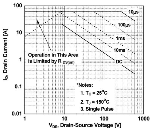
**Figure 10. Maximum Safe Operating Area for FCPF22N60NT**
