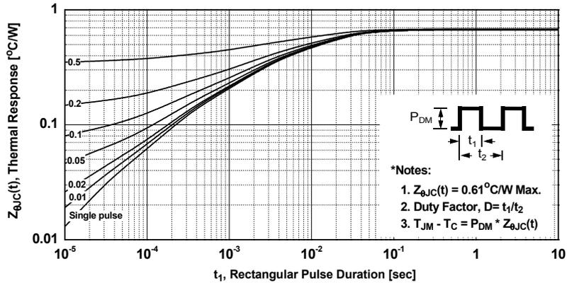
Figure 13. Transient Thermal Response Curve for FCPF22N60NT
