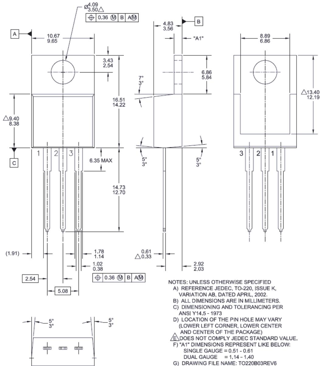
**Figure 18. TO-220, Molded, 3-Lead, Jedec Variation AB**
