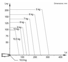
The KR 10 R1100-2 is designed for a rated payload of 5 kg in order to optimize the dynamic performance of the robot. With reduced load center distances, higher loads up to the maximum payload may be used. The specific load case must be verified using KUKA.Load. For further consultation, please contact KUKA Support.
