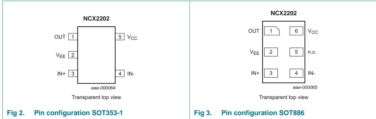
Fig 2. Pin configuration SOT353-1
