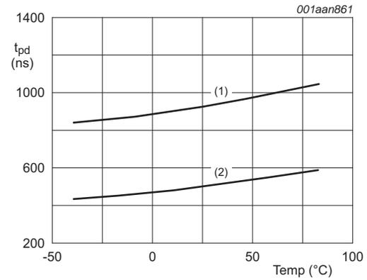
$V_{CC} = 5.0\text{ V}$ ; input overdrive = 50 mV.
