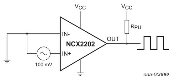
Fig 12. Zero-crossing detector
