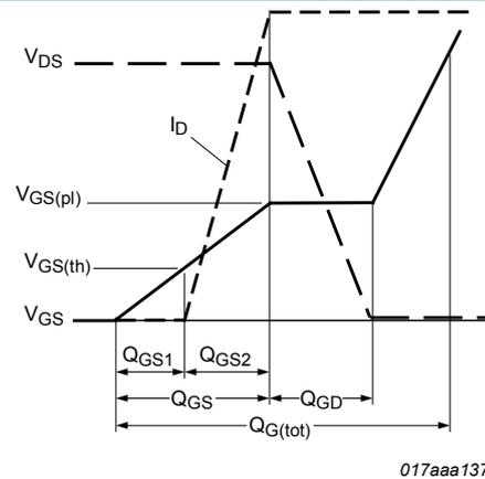
Fig. 15. MOSFET transistor: Gate charge waveform definitions
