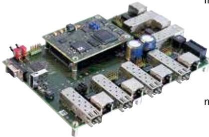
In addition, the EES25 supports precise synchronization as per IEEE 1588v2, plus PRP (Parallel Redundancy Protocol) and HSR (High-availability Seamless Redundancy Protocol), which guarantee uninterrupted data communication. Both versions can be integrated into the Hirschmann network management software Industrial HiVision.
