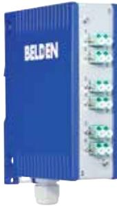
MIPP Fiber Splice Box guarantees efficient fiber termination and is designed for use in a wide range of industrial applications. MIPP Fiber Splice Box accommodates various fiber types and connectors: LC, SC, SC metal, ST, ST metal and E-2000 fiber duplex adapters.
