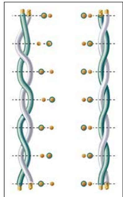
**Illustration 3:** Side-by-side comparison. Non-Bonded-Pair versus Bonded-Pair cable.
