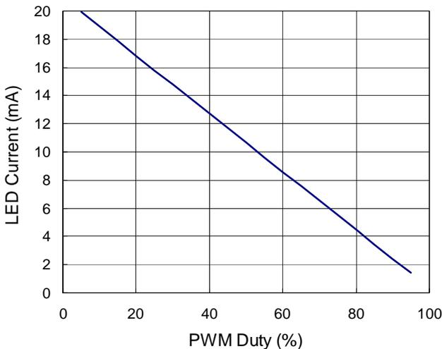
Figure 4. PWM Duty Cycle vs. LED Current
