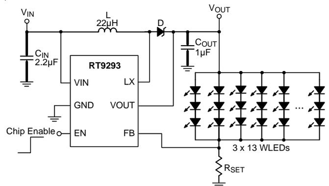
Figure 6. Application for Driving 3 X 13 WLEDs
