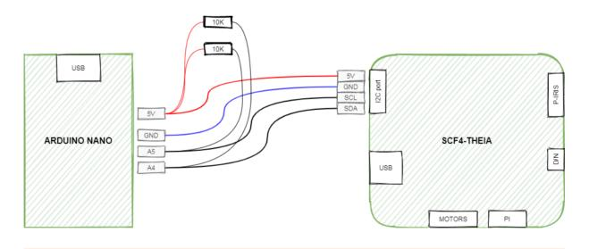
In order to avoid power loops, do not connect both (SCF4 and Arduino) USB ports at the same time.
