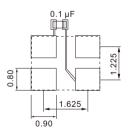
To ensure optimal oscillator performance, place a by-pass capacitor of 0.1  $\mu F$  as close to the part as possible between Vdd and GND pads.
