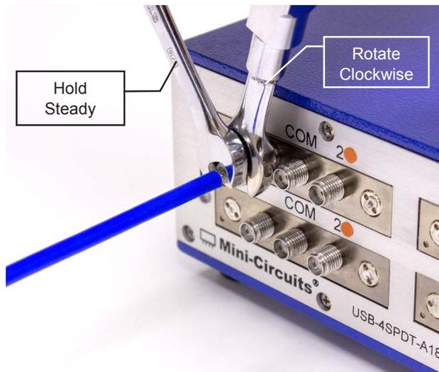
**\*NOTE:** Mini-Circuits recommends using a 5/16-inch open end wrench calibrated to 8 inch-pounds maximum torque to prevent damage due to over-torquing the connector.
