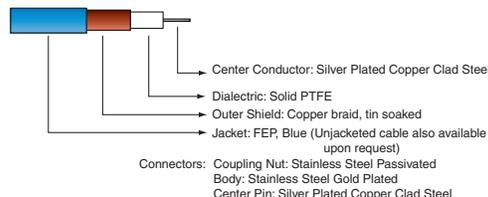
Connectors: Coupling Nut: Stainless Steel Passivated
