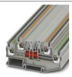
Feed-through terminal block, Cross section: 0.14 mm<sup>2</sup> - 4 mm<sup>2</sup>, AWG: 26 - 12, Connection type: Push-in connection, Width: 5.2 mm, Color: gray, Mounting type: NS 35/7,5, NS 35/15
