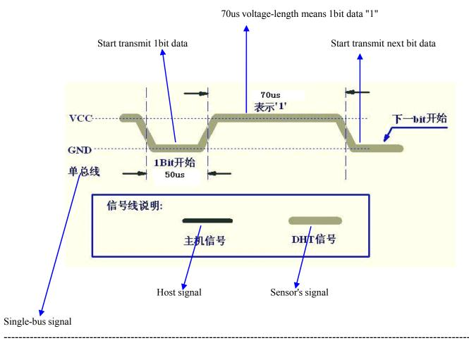
If signal from AM2303 is always high-voltage-level, it means AM2303 is not working properly, please check the electrical connection status.
