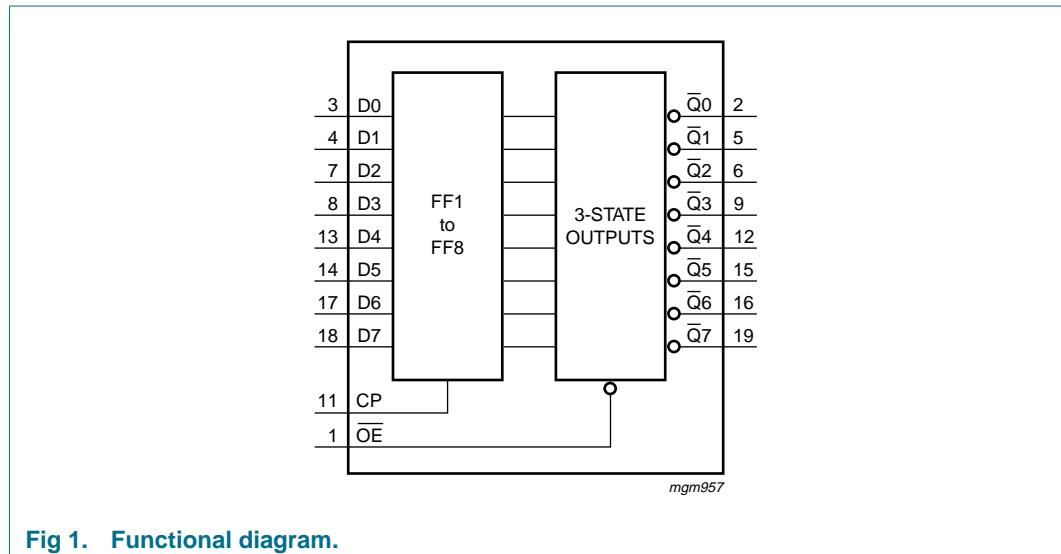
**Fig 1. Functional diagram.**
