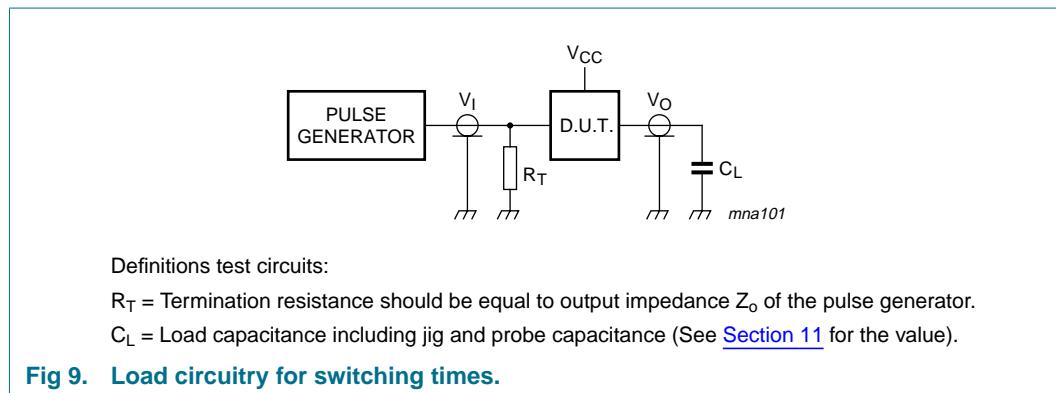
Fig 9. Load circuitry for switching times.
