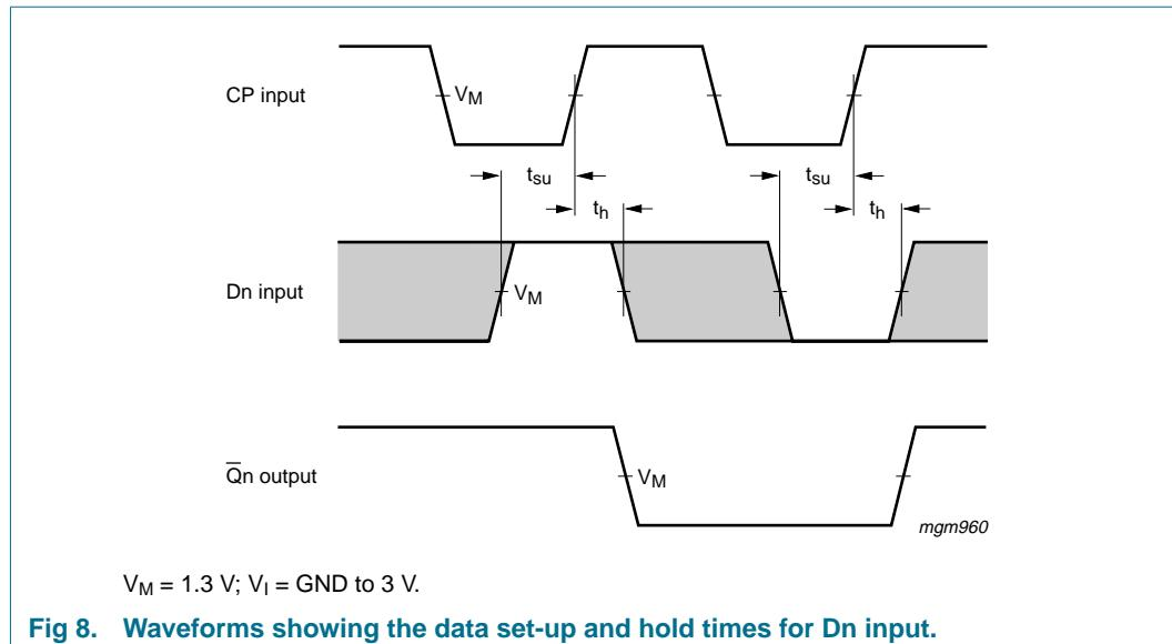
Fig 8. Waveforms showing the data set-up and hold times for D<sub>n</sub> input.
