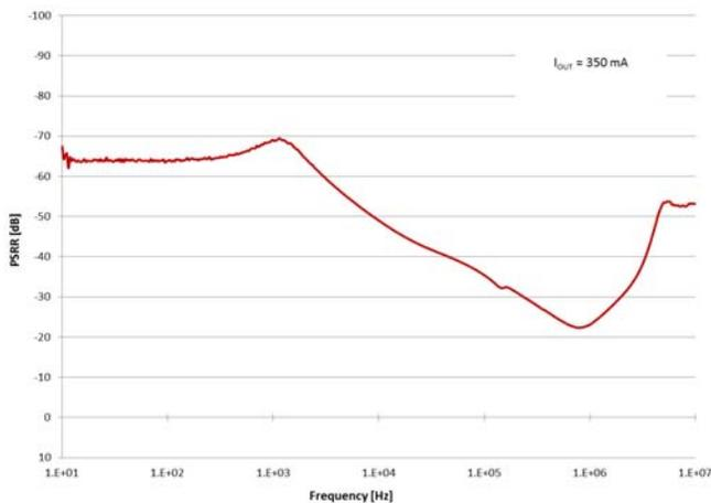
Figure 14.  $V_{BIAS}$  Power Supply Ripple Rejection vs. Frequency
