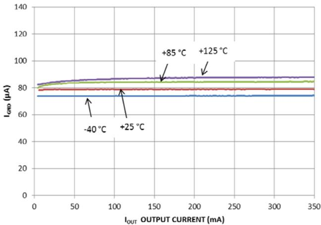
Figure 8. Bias Pin Current vs. Output Current
