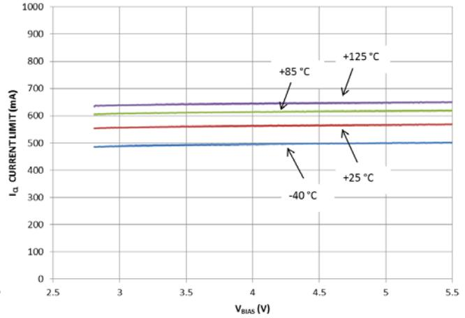
Figure 11. Current Limit vs.  $V_{BIAS}$  Input Voltage
