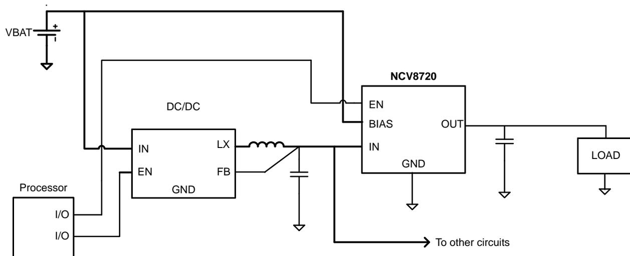
Figure 3. Typical Application: Low-Voltage Post-Regulator with ON/OFF functionality
