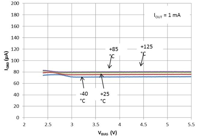
Figure 7. Bias Pin Current vs.  $V_{BIAS}$  Input Voltage
