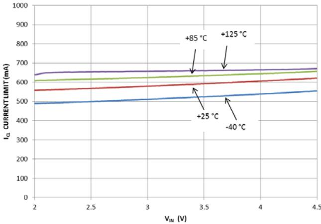
Figure 12. Current Limit vs.  $V_{IN}$  Input Voltage
