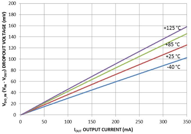
Figure 4.  $V_{IN}$  Dropout Voltage vs. Output Current
