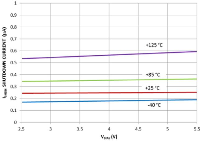
Figure 10. Shutdown Current vs.  $V_{BIAS}$  Input Voltage
