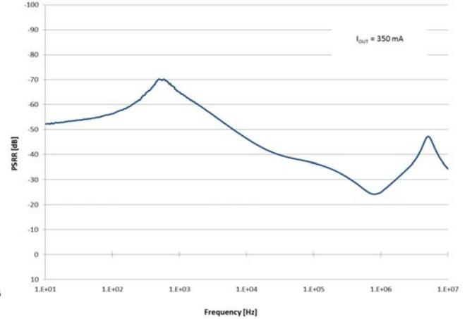
Figure 13.  $V_{IN}$  Power Supply Ripple Rejection vs. Frequency
