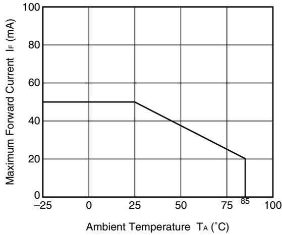
**MAXIMUM LOAD CURRENT vs. AMBIENT TEMPERATURE**
