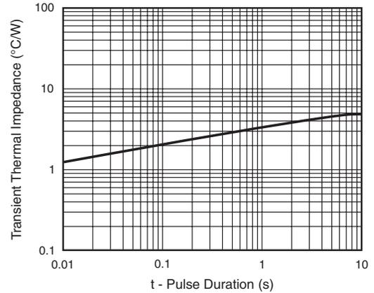
Figure 5. Typical Transient Thermal Impedance Per Diode
