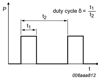
Fig. 13. Duty cycle definition
